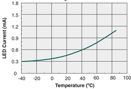
Typical  $I_F$  for Switch Dropout
