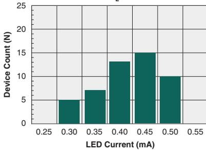
Typical I<sub>F</sub> for Switch Dropout
