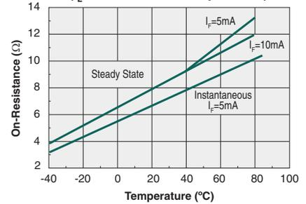
Typical  $I_F$  for Switch Operation
