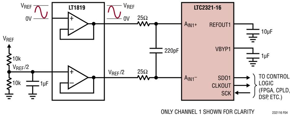
Figure 4. Pseudo-Differential Bipolar Application Circuit
