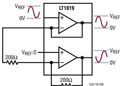
Figure 8. Single-Ended to Differential Driver
