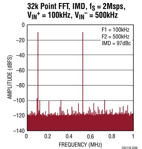
**TYPICAL PERFORMANCE CHARACTERISTICS**  $T_A = 25^\circ\text{C}$ ,  $V_{DD} = 5\text{V}$ ,  $OV_{DD} = 2.5\text{V}$ ,  $REF_{OUT1,2} = 4.096\text{V}$ ,  $f_{SAMPL} = 2\text{Msps}$ , unless otherwise noted.
