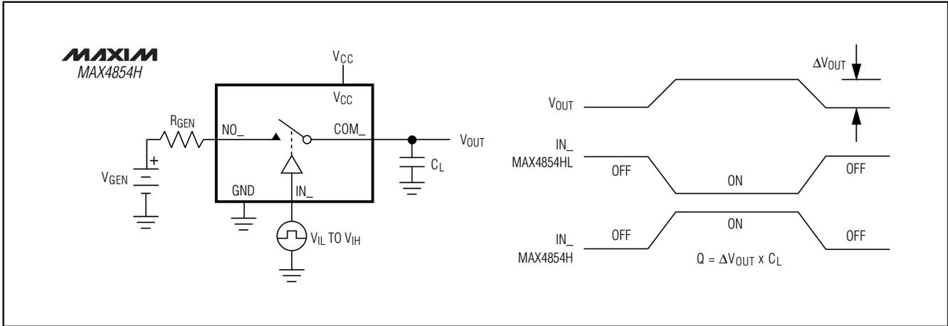
Figure 3. Charge Injection
