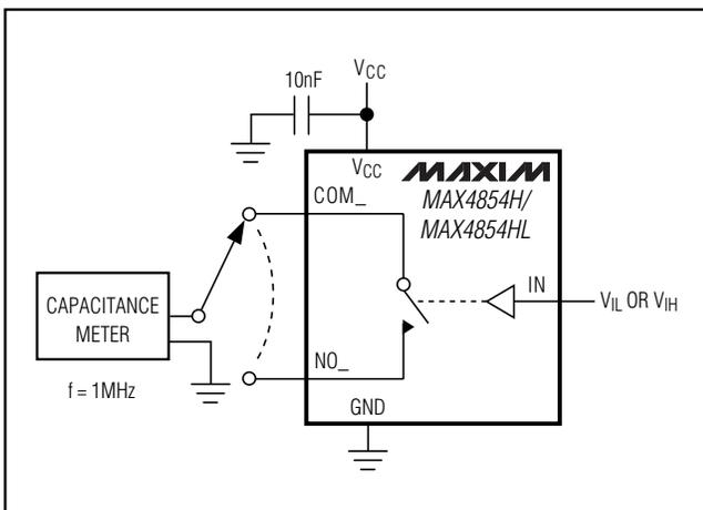
Figure 5. Channel Off-/On-Capacitance
