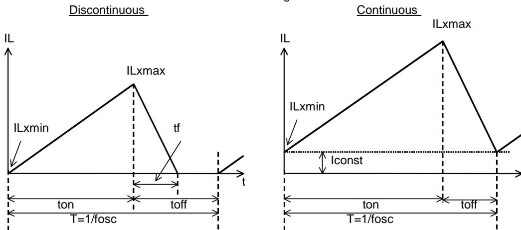
There are two modes, or discontinuous mode and continuous mode for the PWM step-up switching regulator depending on the continuous characteristic of inductor current. During on time of the transistor, when the voltage added on to the inductor is described as  $V_{IN}$ , the current is  $V_{IN} \times t / L$ . Therefore, the electric power,  $P_{ON}$ , which is supplied with input side, can be described as in next formula.
