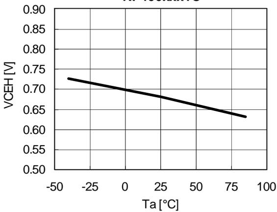
12) Feedback Voltage vs. Temperature
