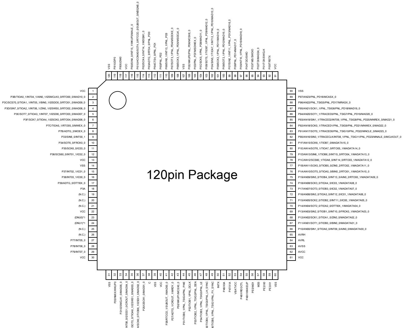
\*1: The DNU0 / 1 (23 pin / 24 pin), please pull up and short-circuit on the board.
