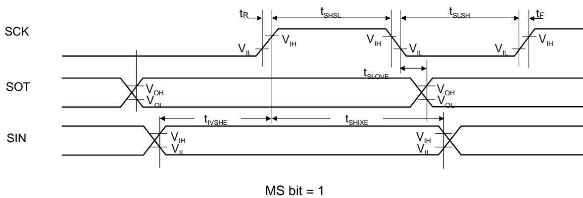
**When Using Synchronous Serial Chip Select (SCINV = 0, CSLVL=1)**
