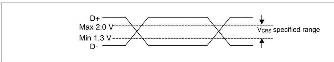
\*5: They indicate Rising time ( $t_{FR}$ ) and Falling time ( $t_{FF}$ ) of the Full-speed differential data signal.
