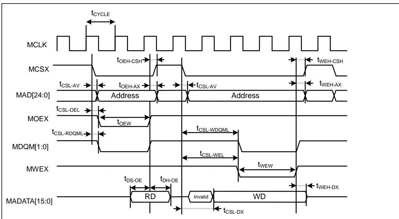
**Separate Bus Access Synchronous SRAM Mode**
