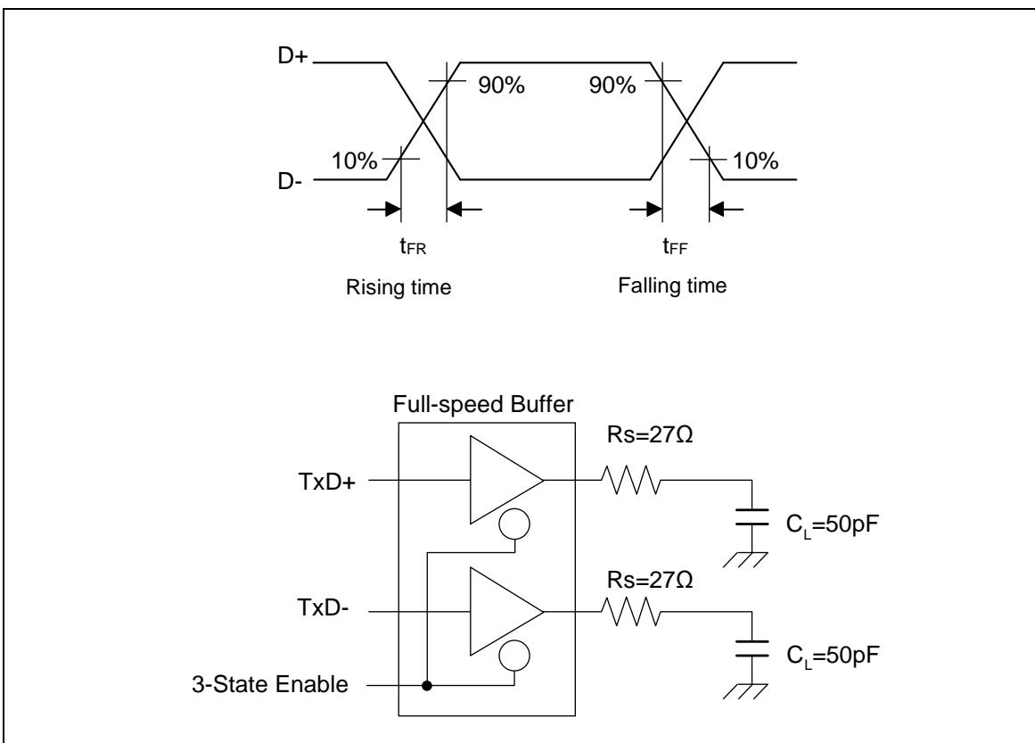
\*6: USB Full-speed connection is performed via twist pair cable shield with  $90\ \Omega \pm 15\%$  characteristic impedance (Differential Mode).
