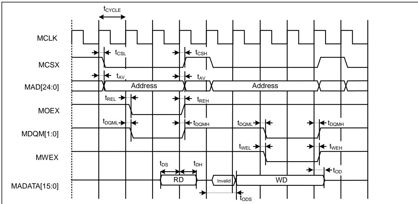
**Multiplexed Bus Access Asynchronous SRAM Mode**
