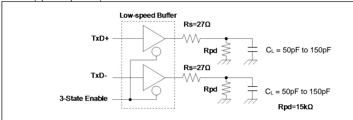
■ Low-speed load (Downstream port load) - Reference 2
