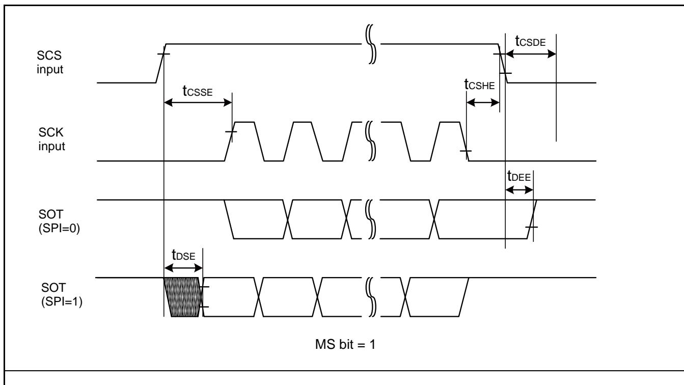
**External Clock (EXT = 1): when in Asynchronous Mode Only**
