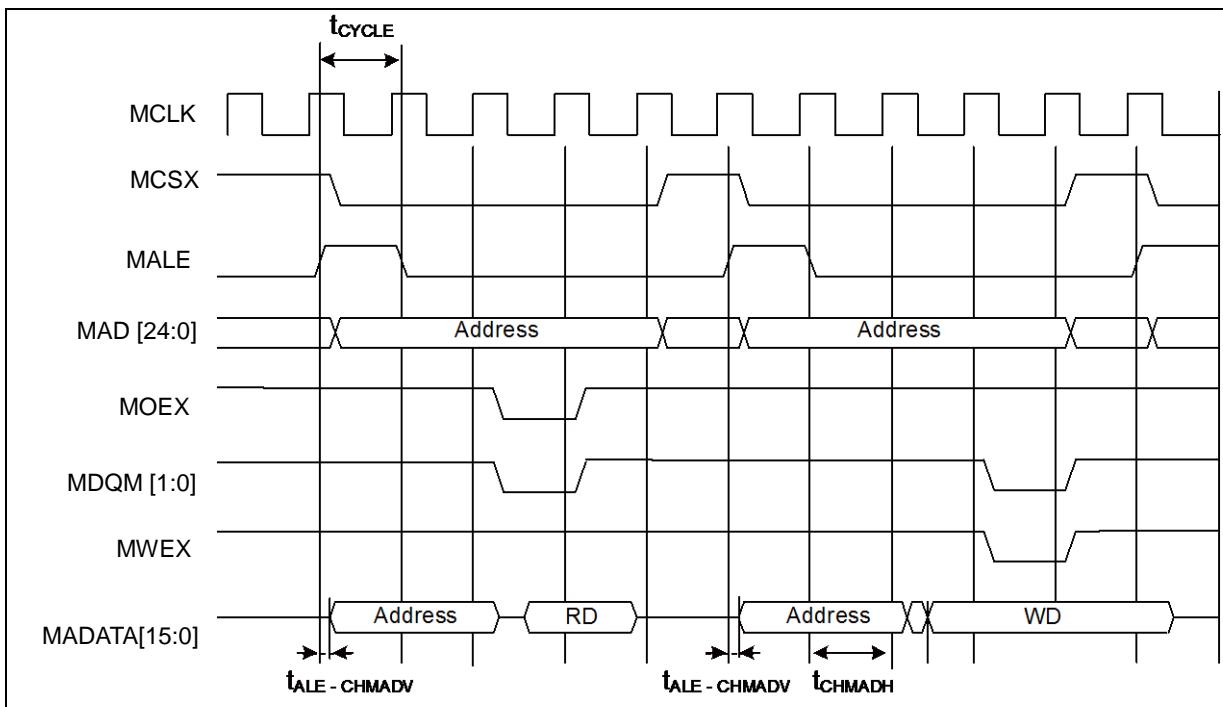
**Multiplexed Bus Access Synchronous SRAM Mode**
