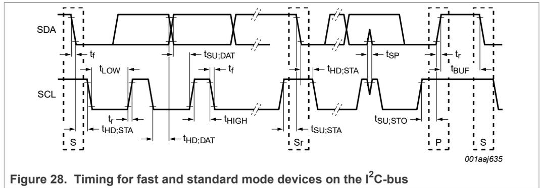
Figure 28. Timing for fast and standard mode devices on the I<sup>2</sup>C-bus
