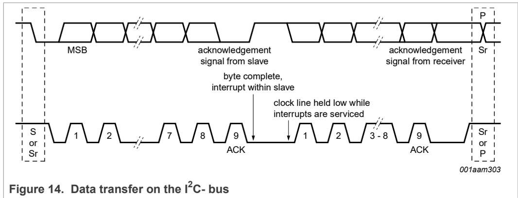
Figure 14. Data transfer on the I<sup>2</sup>C-bus
