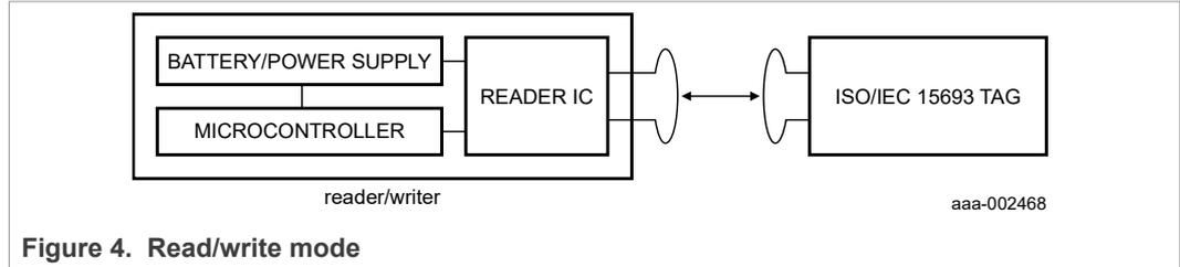
A typical system using the SLRC610 is using a microcontroller to implement the higher levels of the contactless communication protocol and a power supply (battery or external supply).
