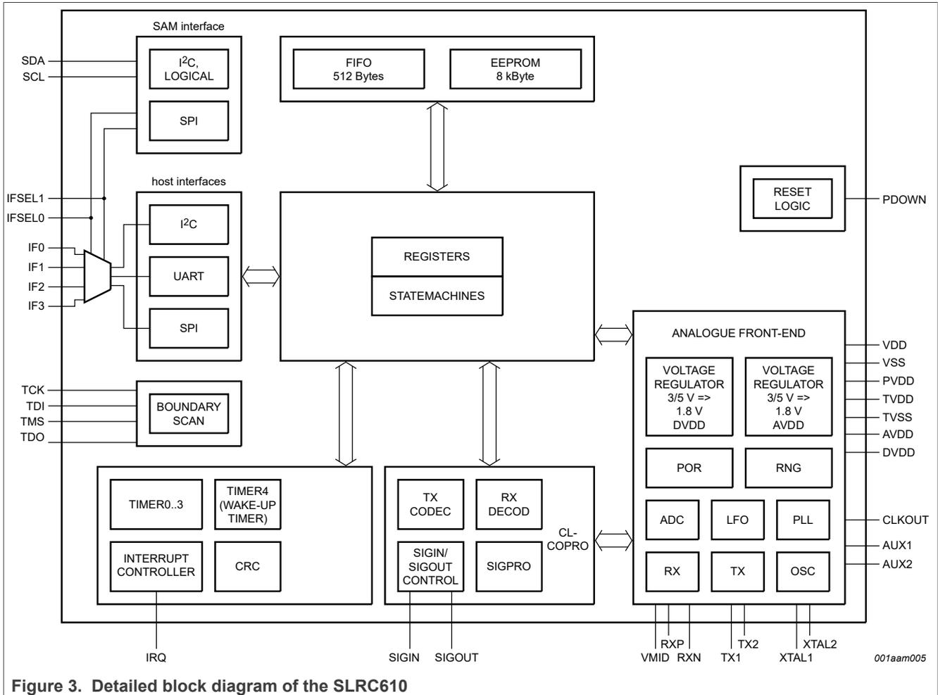
Figure 3. Detailed block diagram of the SLRC610
