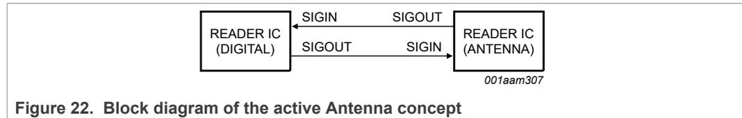
Figure 22. Block diagram of the active Antenna concept
