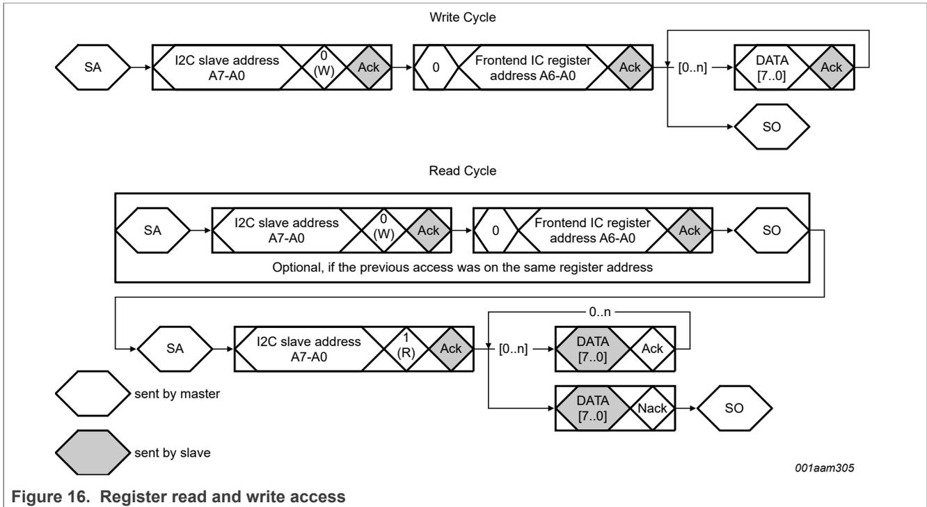
Figure 16. Register read and write access
