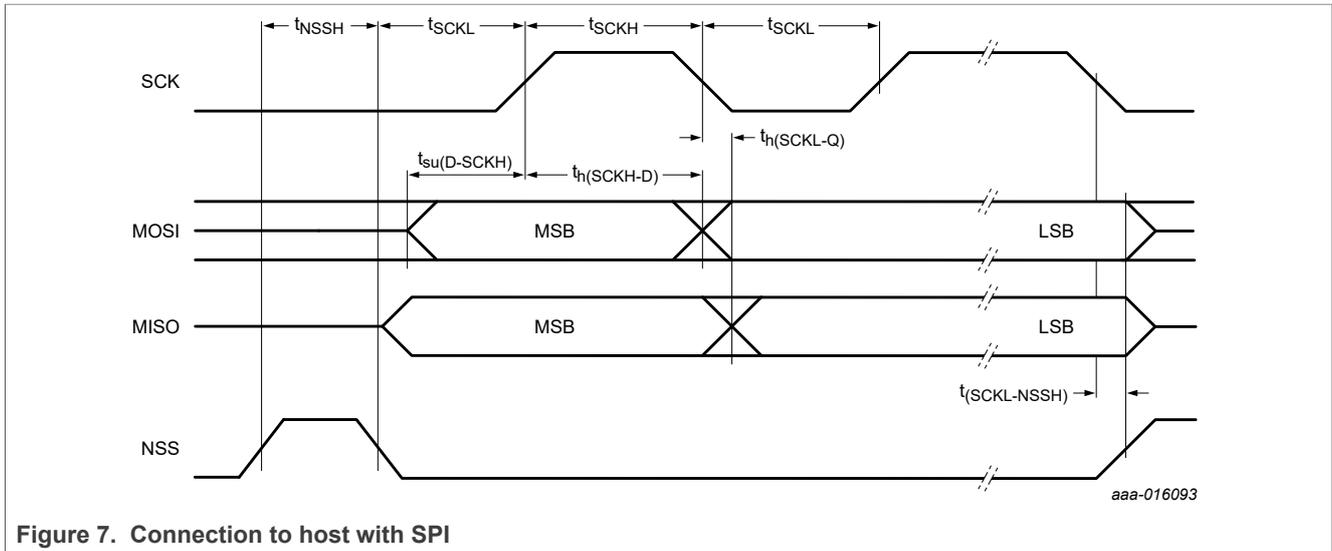
Figure 7. Connection to host with SPI
