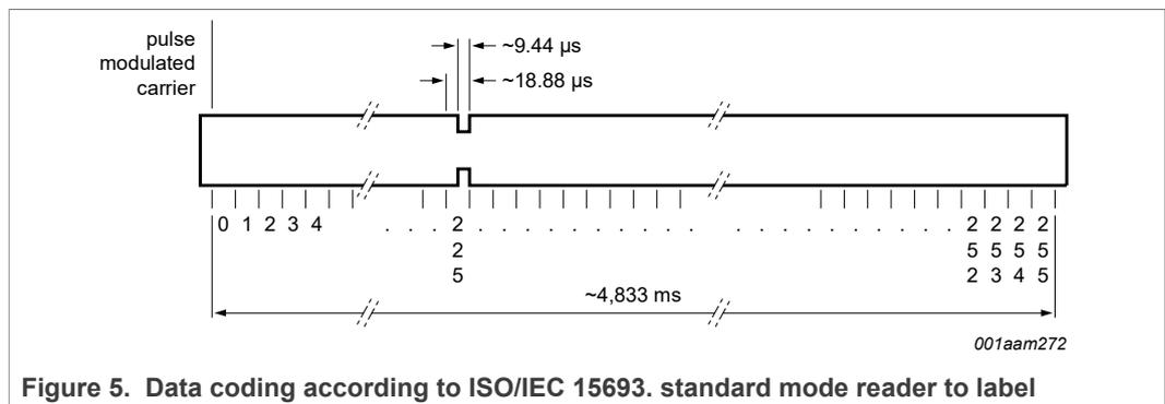
Figure 5. Data coding according to ISO/IEC 15693. standard mode reader to label
