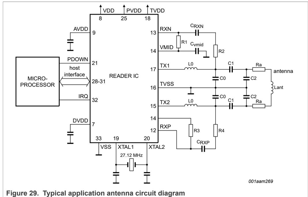
Figure 29. Typical application antenna circuit diagram
