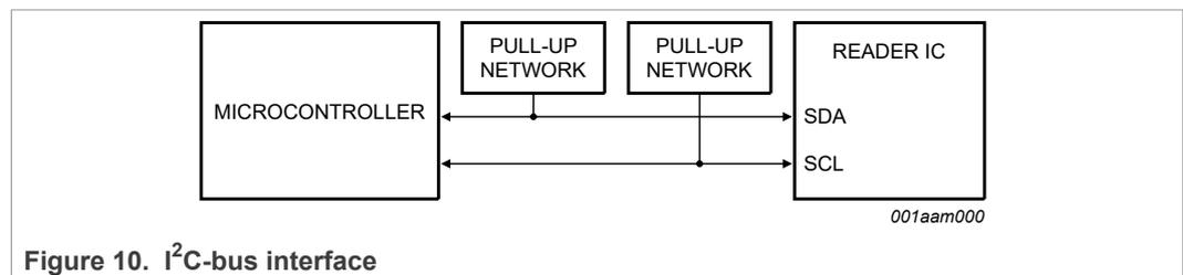
Figure 10. I<sup>2</sup>C-bus interface
