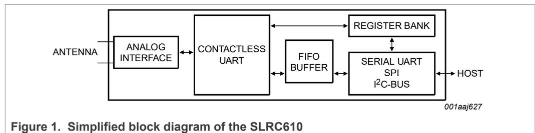
**Figure 1. Simplified block diagram of the SLRC610**
