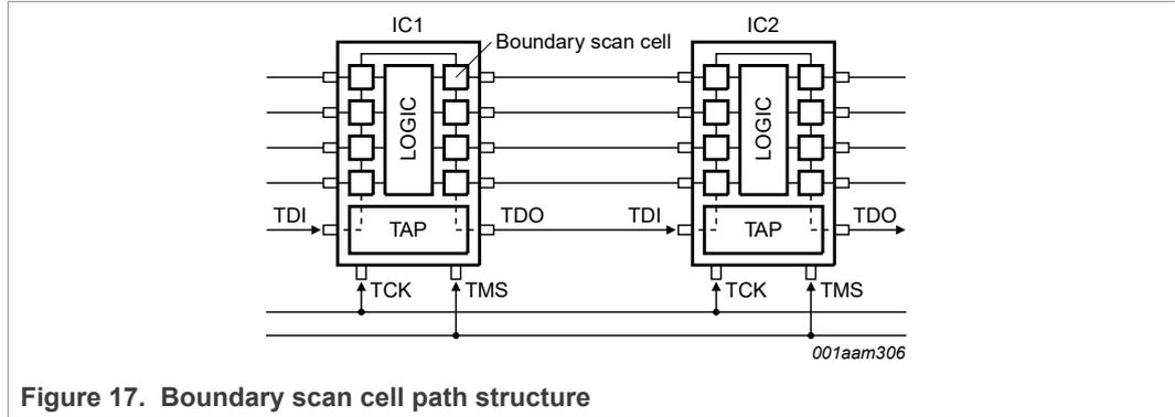
Figure 17. Boundary scan cell path structure
