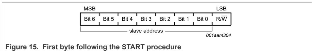
Figure 15. First byte following the START procedure
