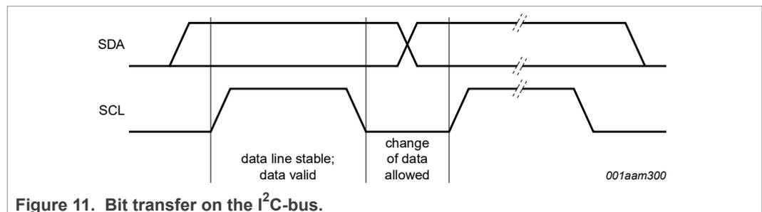
Figure 11. Bit transfer on the I<sup>2</sup>C-bus.
