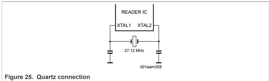
Figure 25. Quartz connection
