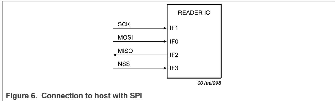
Figure 6. Connection to host with SPI
