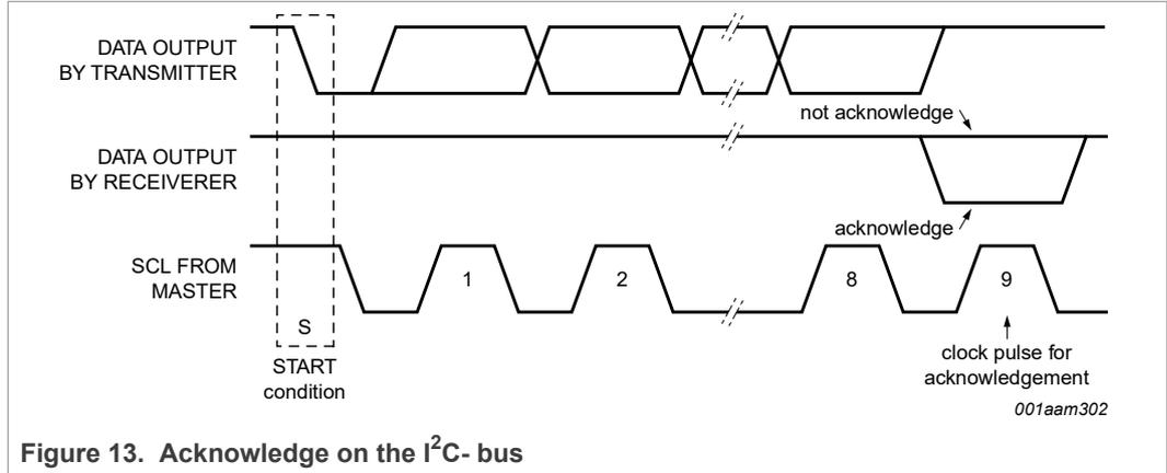
Figure 13. Acknowledge on the I<sup>2</sup>C-bus
