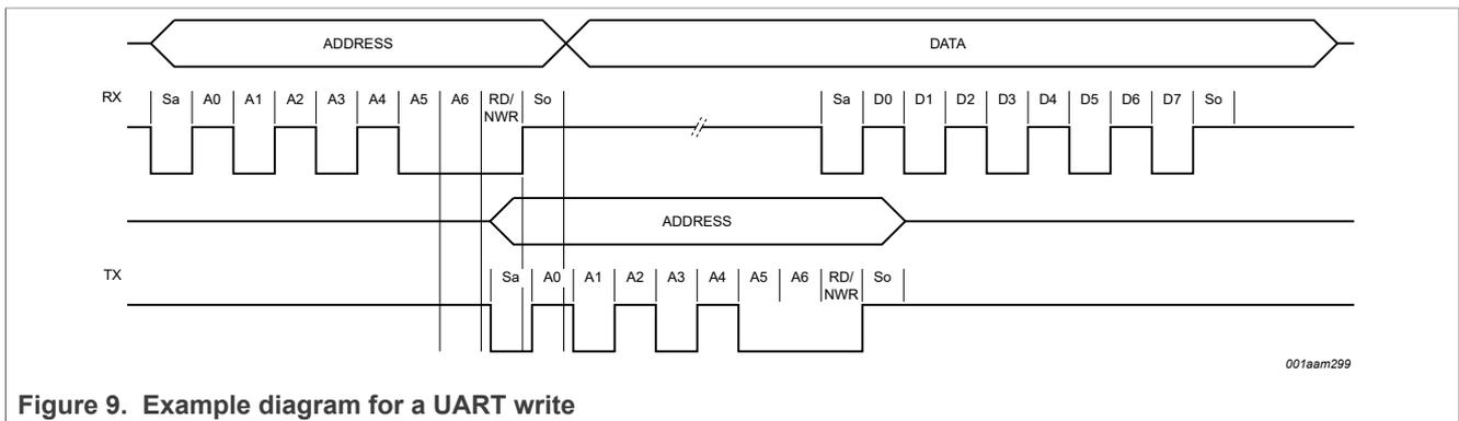
Figure 9. Example diagram for a UART write
