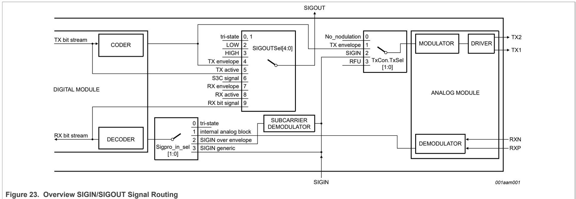
Figure 23. Overview SIGIN/SIGOUT Signal Routing
