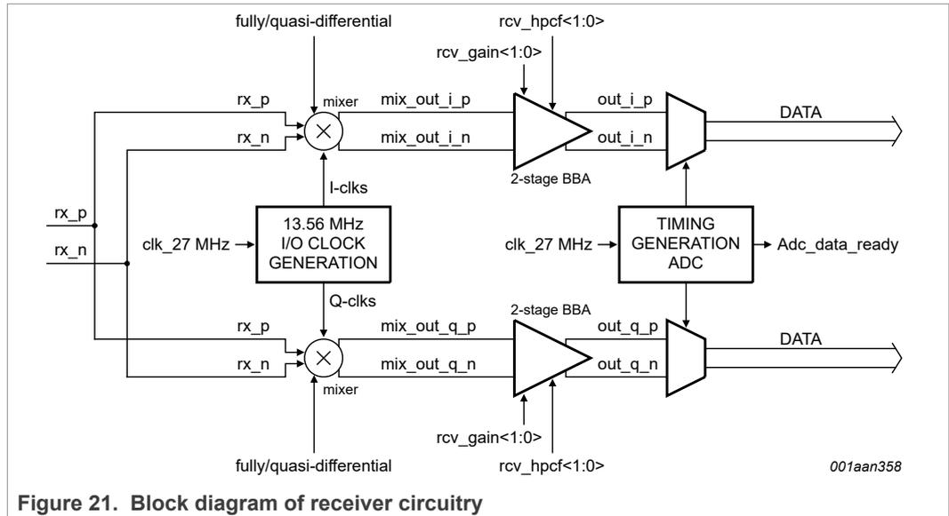
Figure 21. Block diagram of receiver circuitry
