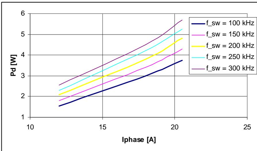
Using the above two diagrams the power loss (= the required power dissipation Pd for thermally stable operation) can be estimated based on a required phase current I<sub>phase</sub> (= current in the Integrated Switch) and based on the switching frequency per phase f<sub>sw</sub> (= frequency of the Integrated Switch in each phase).
