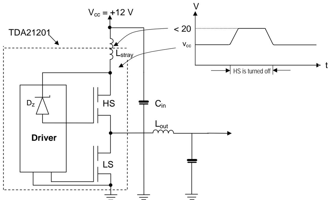
This equation reveals that  $L_{stray}$  should be made as small as possible (as  $v_{cc}(t)$  is limited by the breakdown voltage of the device,  $V_{cc}$  is given by the application,  $di/dt$  should be as large as possible to reduce switching losses) using proper layout techniques and low ESL capacitors, e.g. ceramics, between the Vcc and GND pins of the Integrated Switch.
