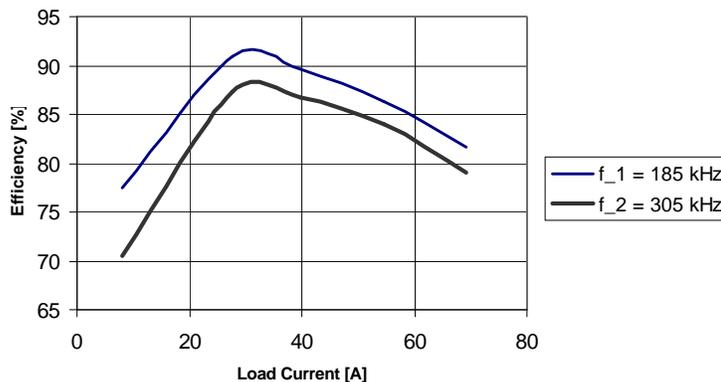
II 4-Phase Converter: Efficiency vs. Switching frequency
