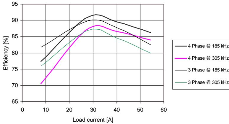
It should be noted that the overall converter efficiency and the maximum converter output power will increase as the output voltage increases, e.g.  $V_O = 2.5$  or  $3.3$  V.
