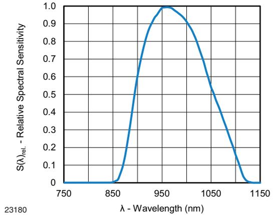
Fig. 10 - Relative Spectral Sensitivity vs. Wavelength
