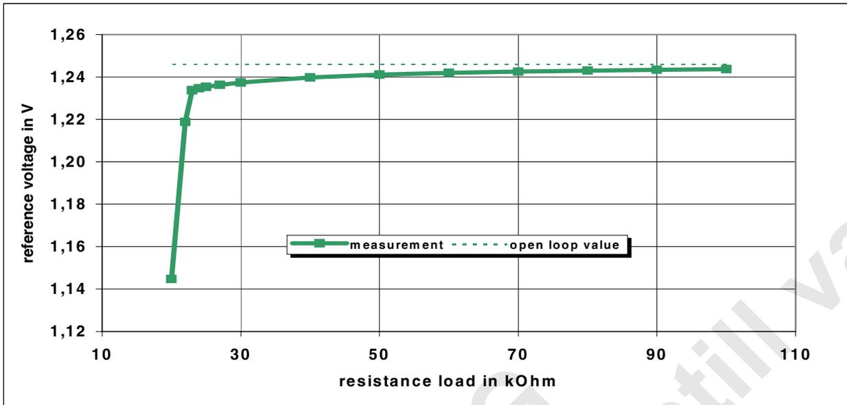
Figure 4: Reference voltage as function of resistance load
