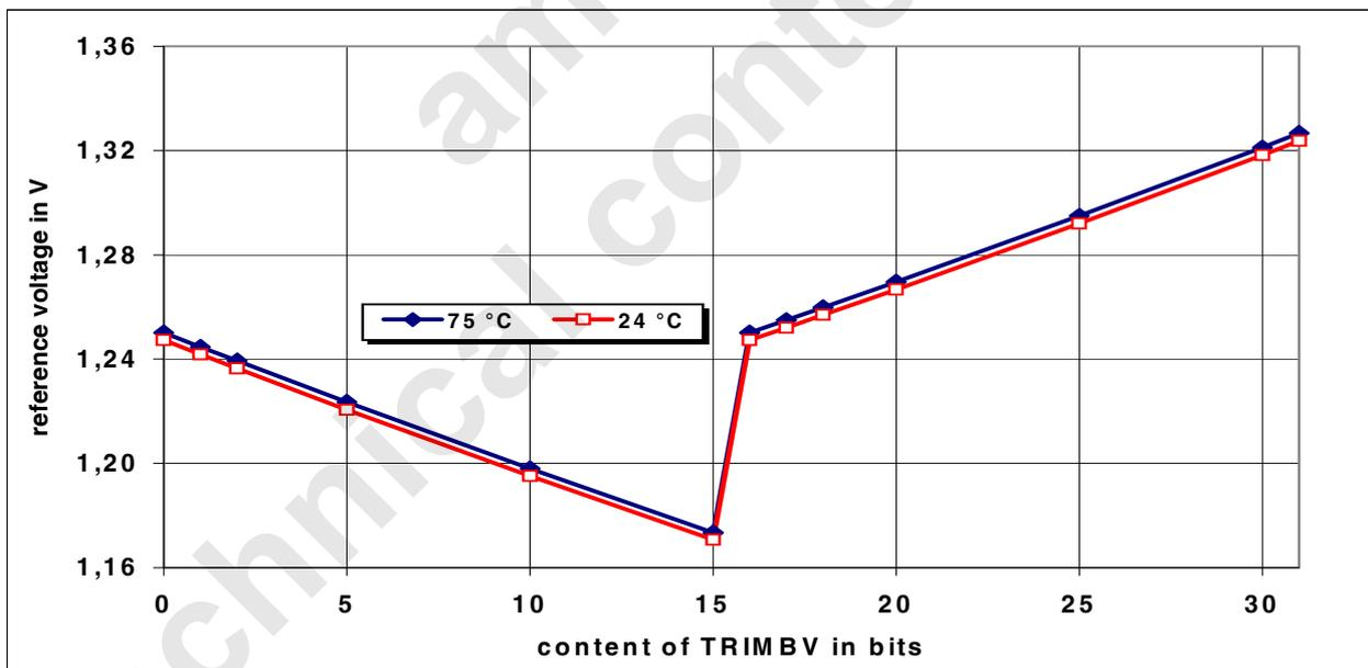
Figure 5: Reference voltage as function of temperature
