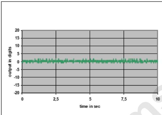
Figure 23: Noise at 125 Hz sampling rate, gain 24
