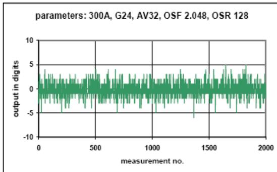
Figure 13: Resolution and noise at zero input, sampling rate: 1kHz
