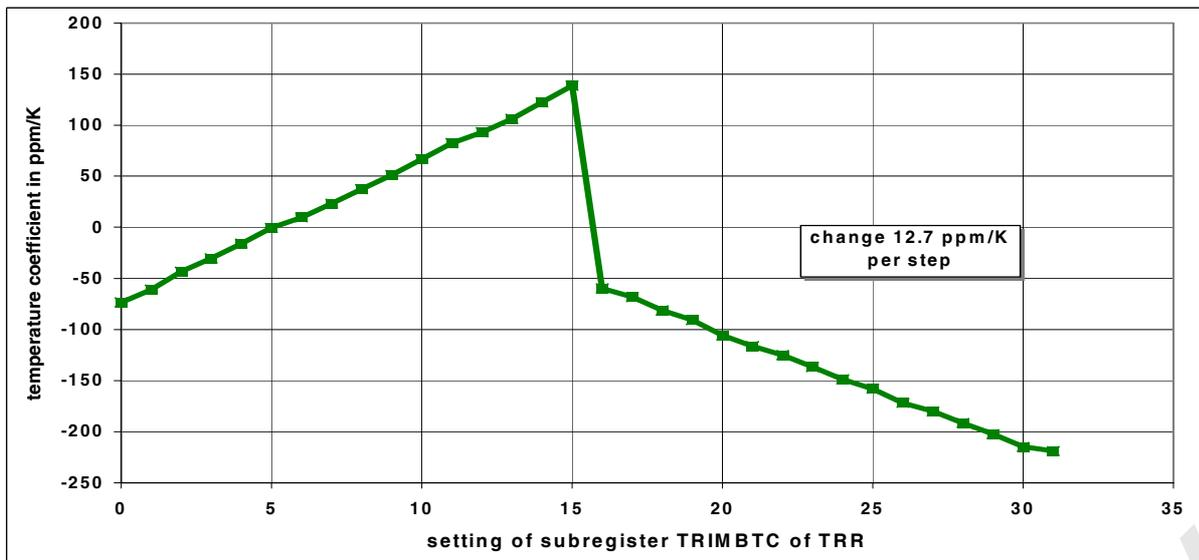
Figure 6: Temperature coefficient as function of TRIMBTC setting
