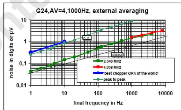
Figure 18: Output voltage noise over sampling rate
