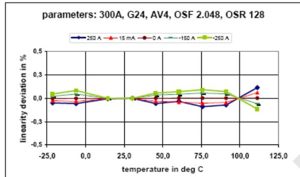
Figure 14: Linearity deviation for different currents over temperature
