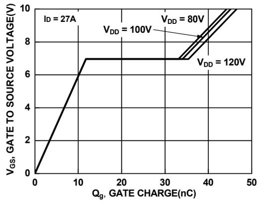
Figure 15. Gate Charge vs. Gate to Source Voltage
