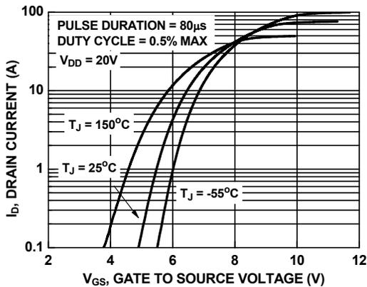
Figure 6. Transfer Characteristics
