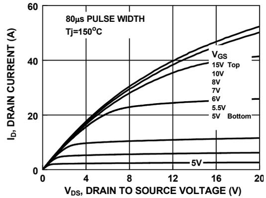
Figure 9. Saturation Characteristics
