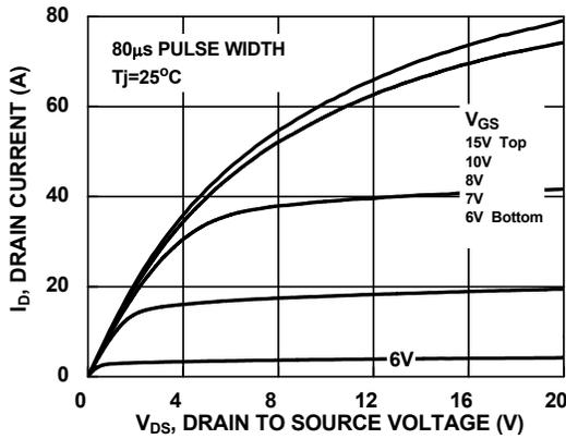
Figure 8. Saturation Characteristics
