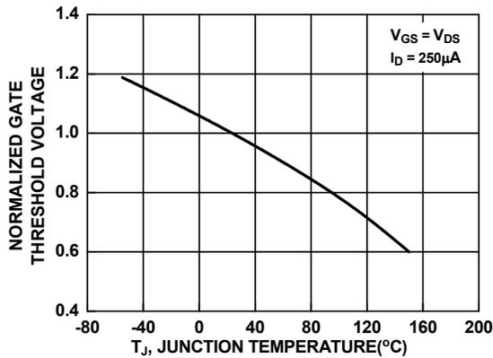
Figure 12. Normalized Gate Threshold Voltage vs. Temperature
