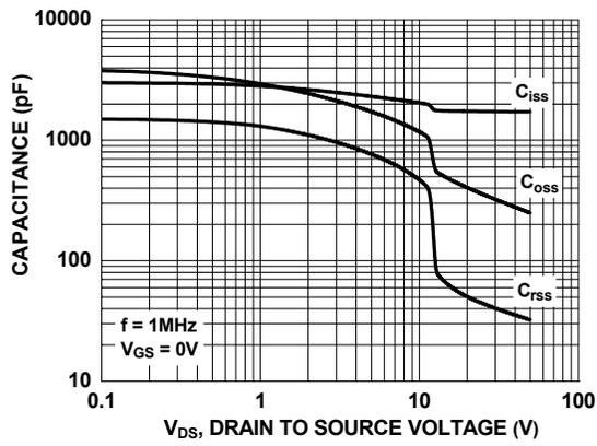
Figure 14. Capacitance vs. Drain to Source Voltage
