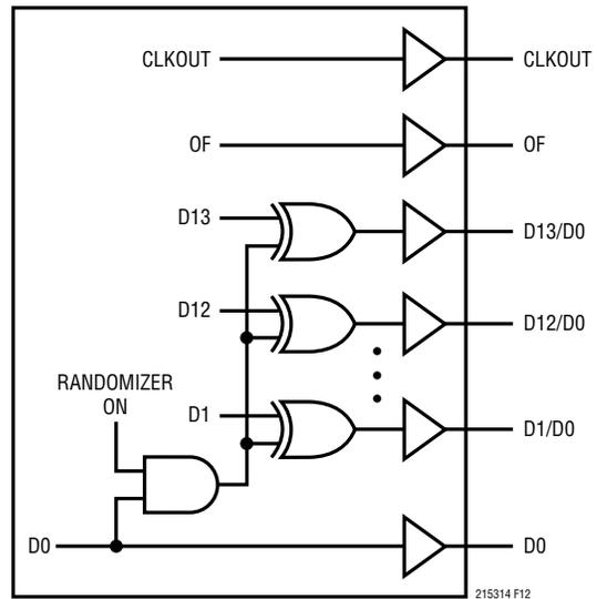
**Figure 12. Functional Equivalent of Digital Output Randomizer**
