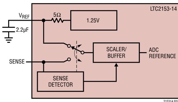
Figure 7. Reference Circuit
