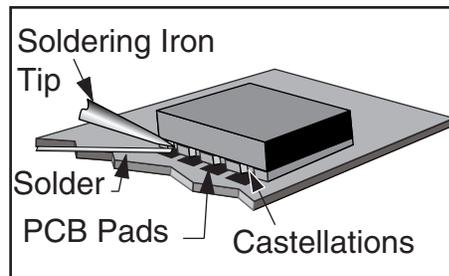
Figure 8: Soldering Technique
