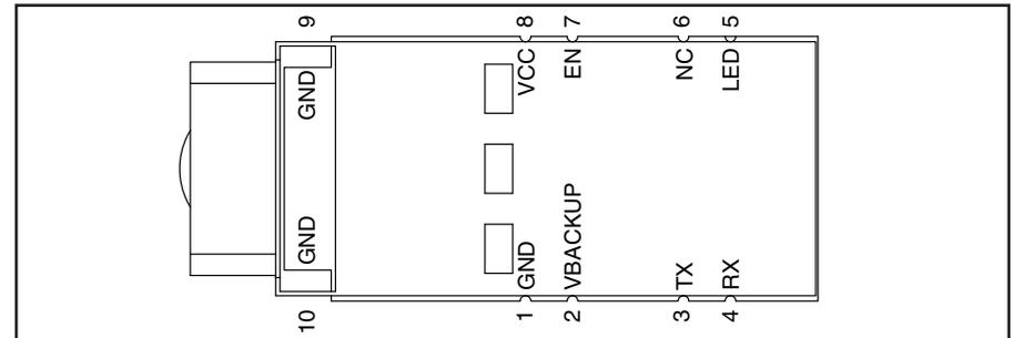
Figure 2: SR Series Receiver Pinout (Top View)
