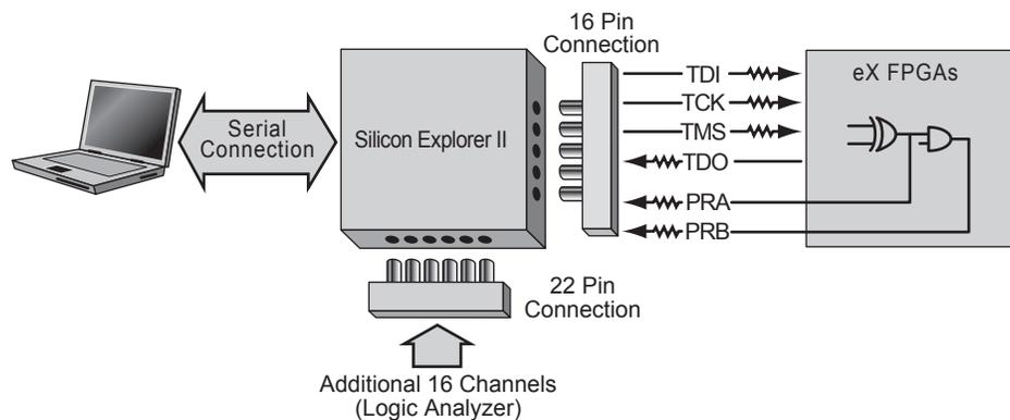
**Figure 1-13 • Silicon Explorer II Probe Setup**
