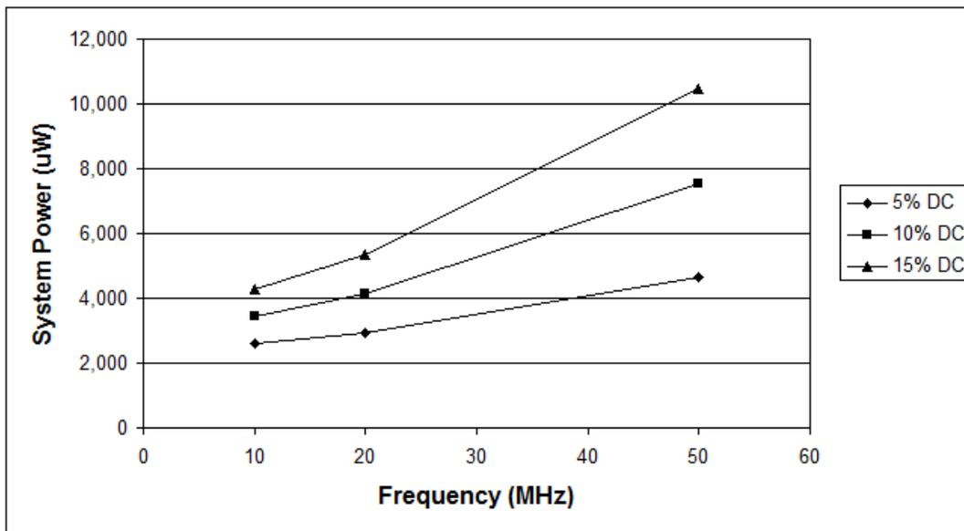
Figure 1-11 • System Power at 5%, 10%, and 15% Duty Cycle
