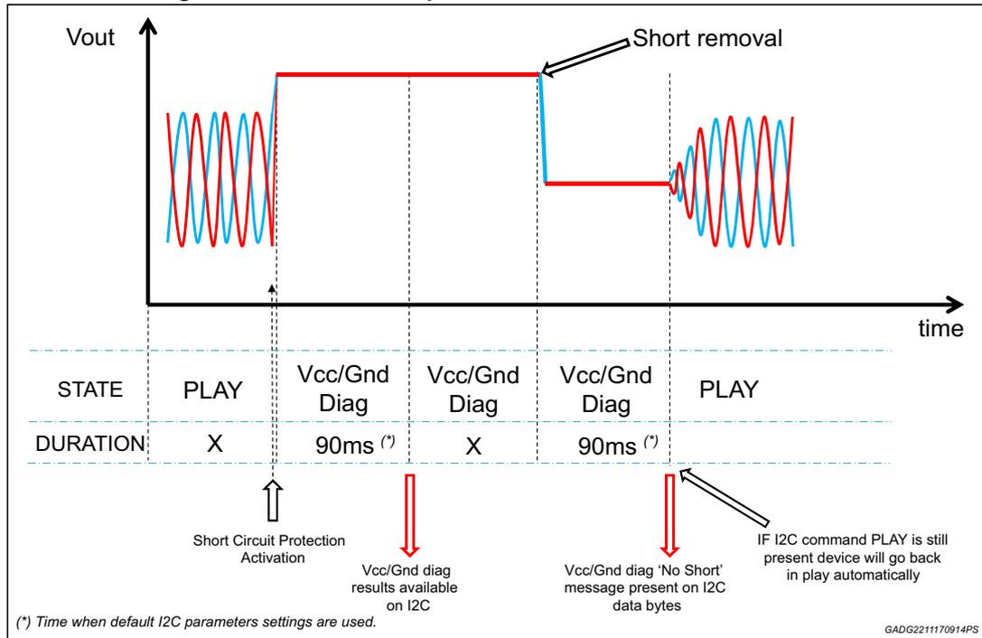
Figure 51. Short Circuit Protection activation due to short across load, short to Vcc/Gnd not present
