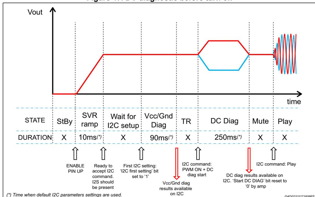
Figure 48. Short to VCC at device turn on
