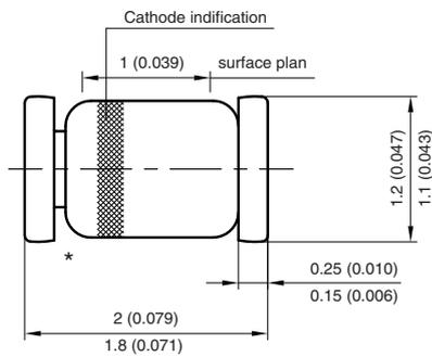
\* The gap between plug and glass can be either on cathode or anode side
