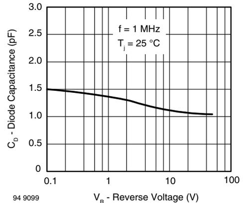
Fig. 4 - Diode Capacitance vs. Reverse Voltage
