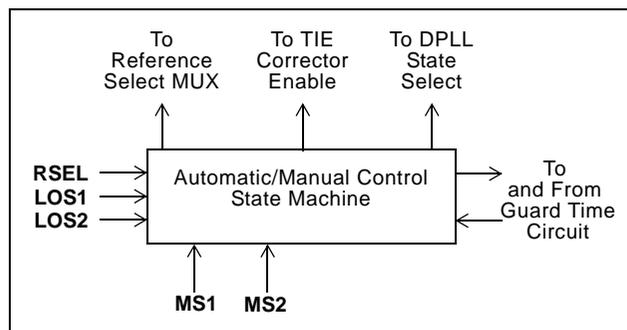
**Figure 6 - Automatic/Manual Control State Machine Block Diagram**
