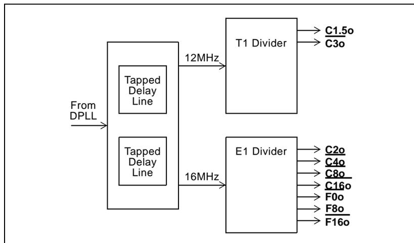
**Figure 5 - Output Interface Circuit Block Diagram**
