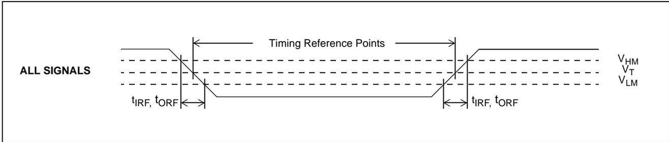
Figure 18 - Timing Parameter Measurement Voltage Levels
