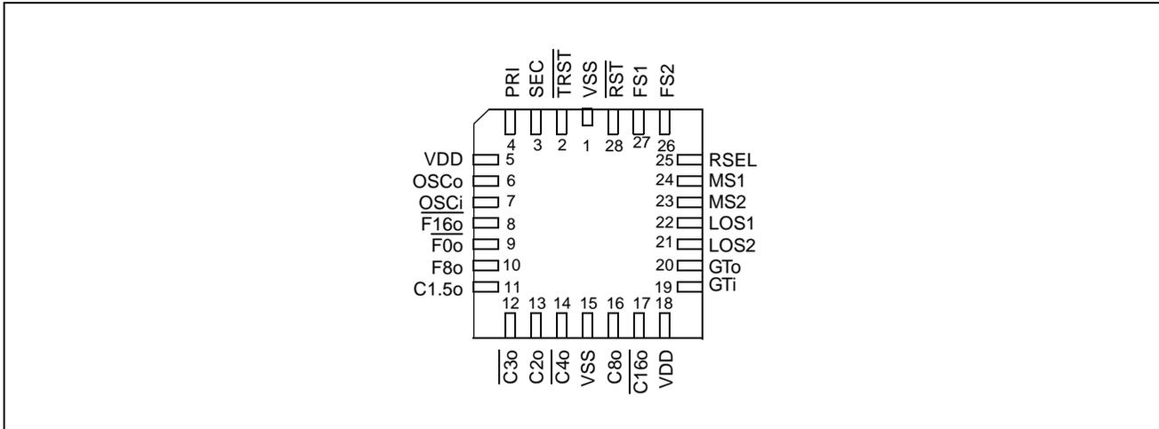
Figure 2 - Pin Connections
