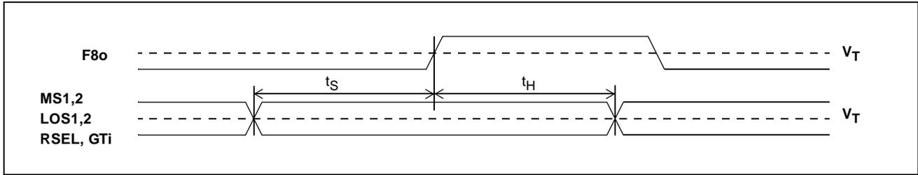
Figure 21 - Input Controls Setup and Hold Timing
