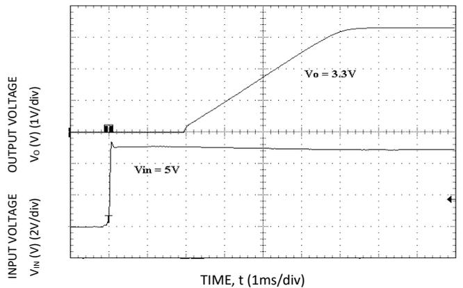
Figure 30. Typical Start-up Using Input Voltage (VIN = 5V, Io = Io,max).
