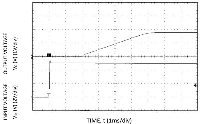
Figure 18. Typical Start-up Using Input Voltage (VIN = 5V, Io = Io,max).
