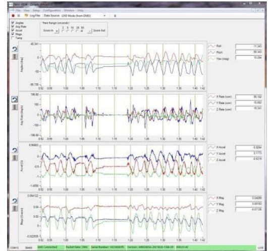
NAV-VIEW provides an easy to use graphical interface to display, record, playback, and analyze all of the IMU380ZA Inertial Measurement System parameters.
