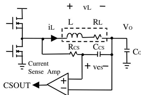
Figure 5. Inductor Current Sensing and Current Sense Amplifier
