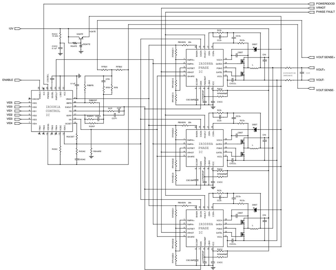
Figure 7. IR3081A/3088A 12V to 2.5V 3 Phase Converter
