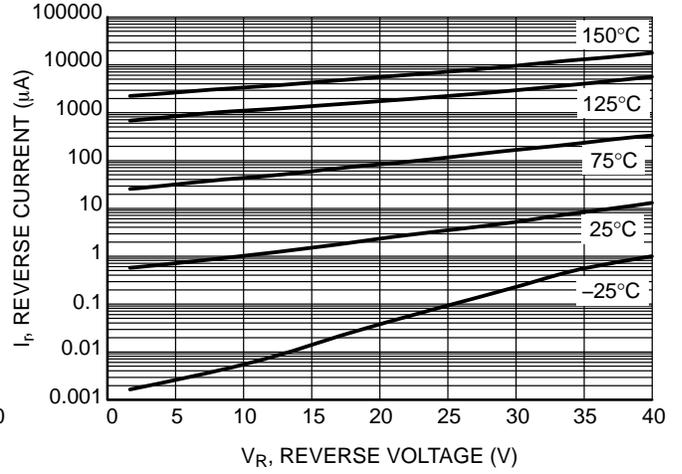
Figure 2. Leakage Current
