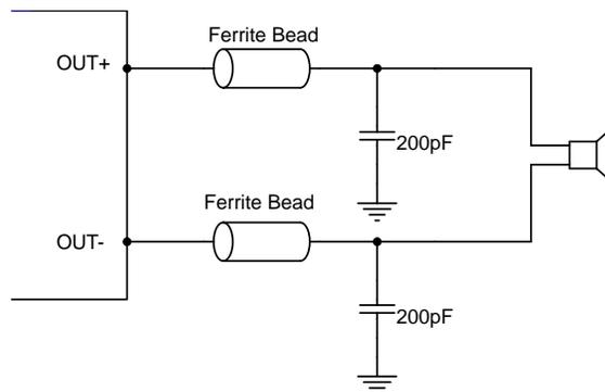
Figure 1. Ferrite Bead Filter to Reduce EMI
