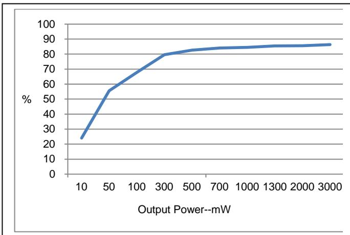
**Efficiency vs. Output Power ( $V_{DD}=5.0\text{V}$ ,  $R_L=8\Omega$ )**
