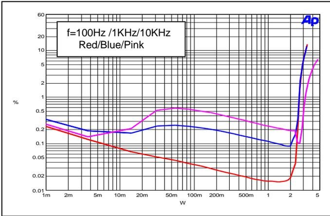
**THD+N vs. Output Power ( $V_{DD}=5\text{V}$ ,  $R_L=8\Omega$ )**
