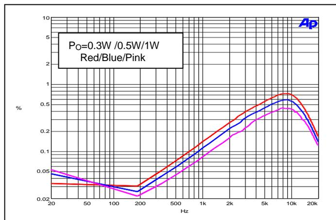
**Performance Characteristics** (@  $T_A = +25^\circ\text{C}$ ,  $V_{DD} = 5\text{V}$ ,  $R_{IN} = 0$ , Gain = 18dB,  $R_L = L(33\mu\text{H})+R+L(33\mu\text{H})$ , unless otherwise specified.)
