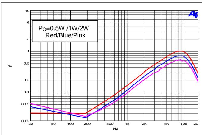
**THD+N vs. Frequency ( $V_{DD}=5.0\text{V}$ ,  $R_L=8\Omega$ )**
