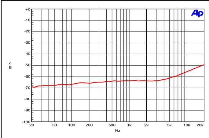
**PSRR vs. Frequency ( $V_{DD}=5.0\text{V}$ ,  $R_L=8\Omega$ )**
