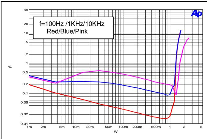
**THD+N vs. Output Power ( $V_{DD}=3.6\text{V}$ ,  $R_L=8\Omega$ )**
