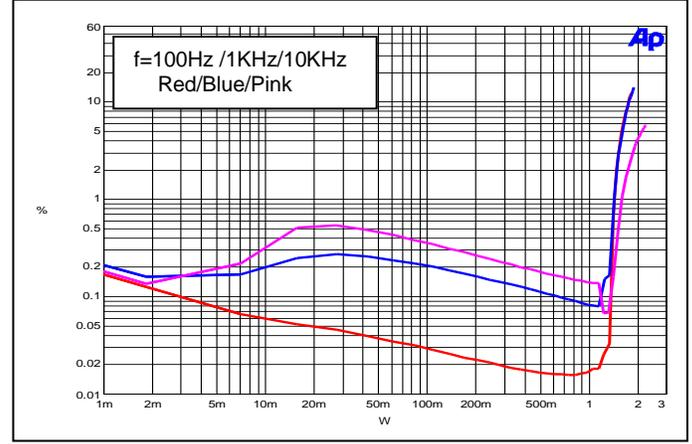
**THD+N vs. Output Power ( $V_{DD}=3.6\text{V}$ ,  $R_L=4\Omega$ )**
