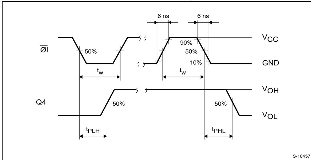
**Figure 6. Waveform 2: propagation delay times, minimum pulse width (CLEAR)
