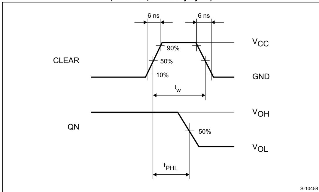
Figure 7. Waveform 3: propagation delay times (f = 1 MHz; 50 % duty cycle)
