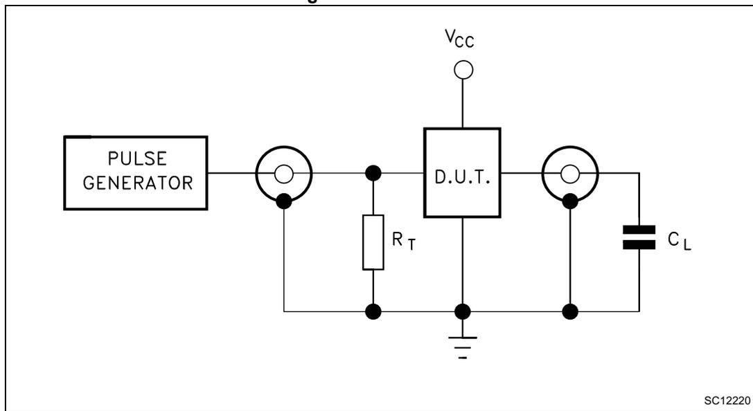
1. C<sub>L</sub> = 50 pF or equivalent (includes jig and probe capacitance)
