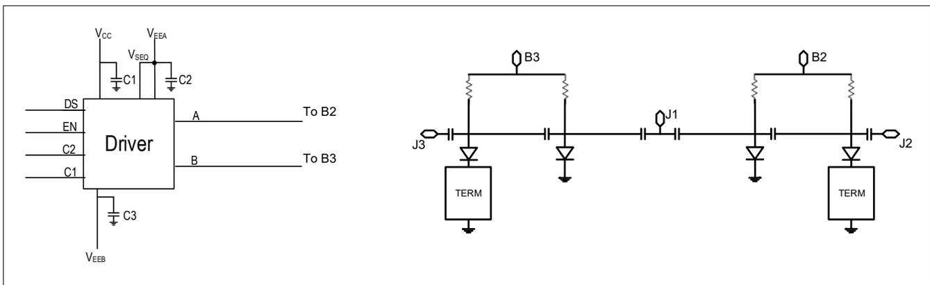
11. Recommended bias with this driver is  $V_{CC} = 5\text{ V}$  and  $V_{EEB} = -30\text{ V}$ .
