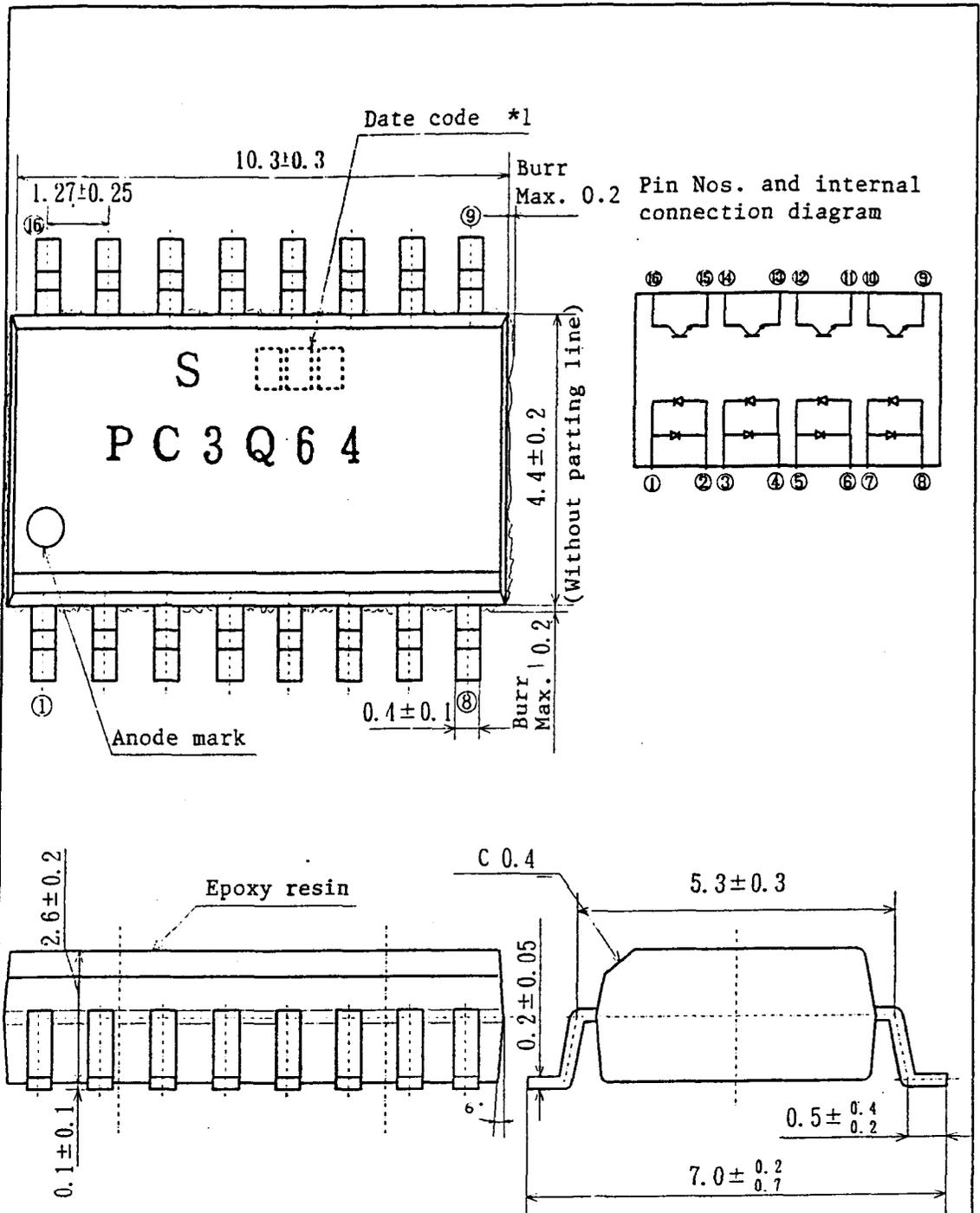
\*1) Date code is composed of 2-digit number marked according to DIN standard and the following weekly code .
