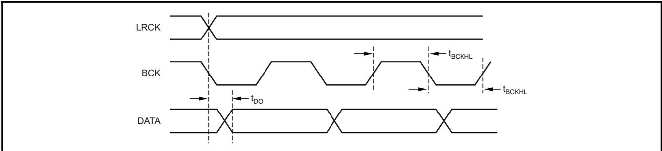
**Figure 1. Audio Serial Port Timing: Left-Justified and I<sup>2</sup>S Data Formats**
