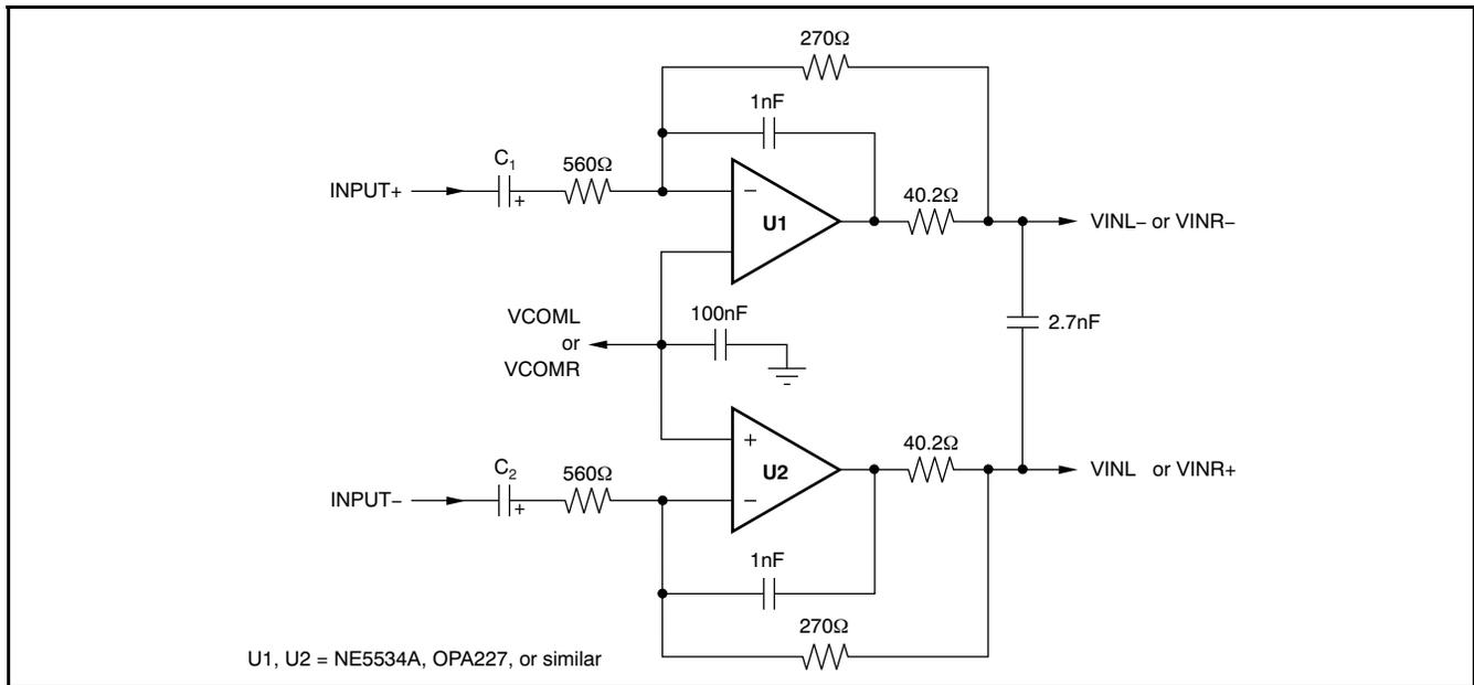
C<sub>1</sub> and C<sub>2</sub> provide ac coupling. They may be removed if the dc offset from the preceding circuit is negligible.
