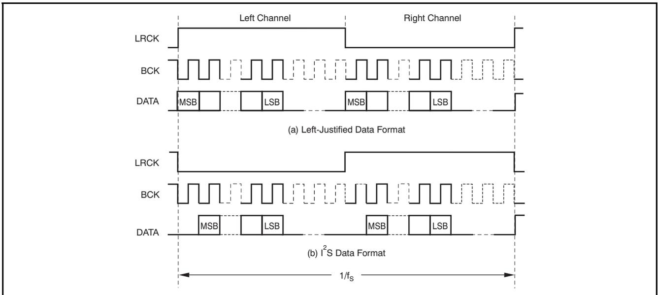
Figure 42. Left-Justified and I<sup>2</sup>S Data Formats
