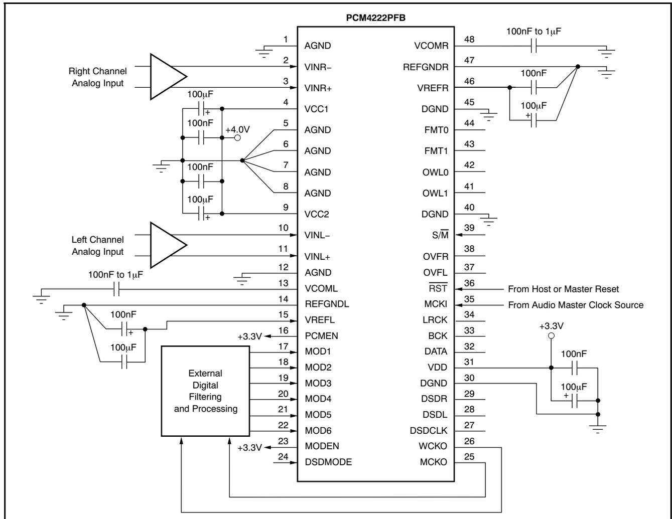
Figure 49. Typical Connections for MBM Output Mode
