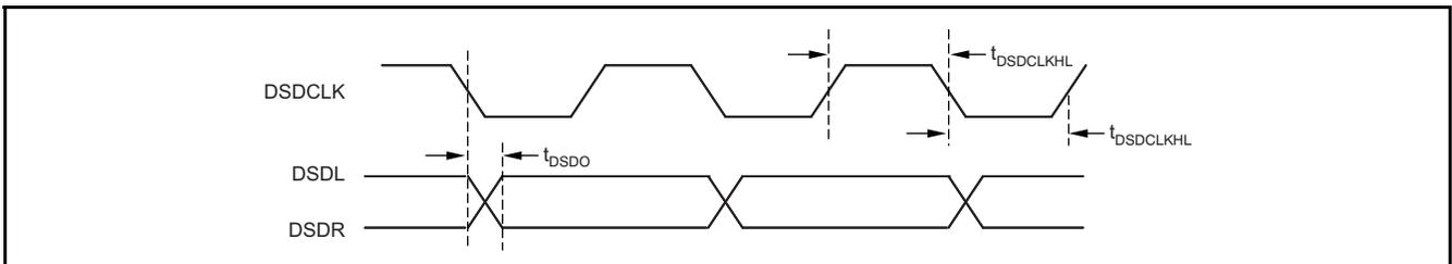
**Figure 3. Direct Stream Digital (DSD) Output Timing**
