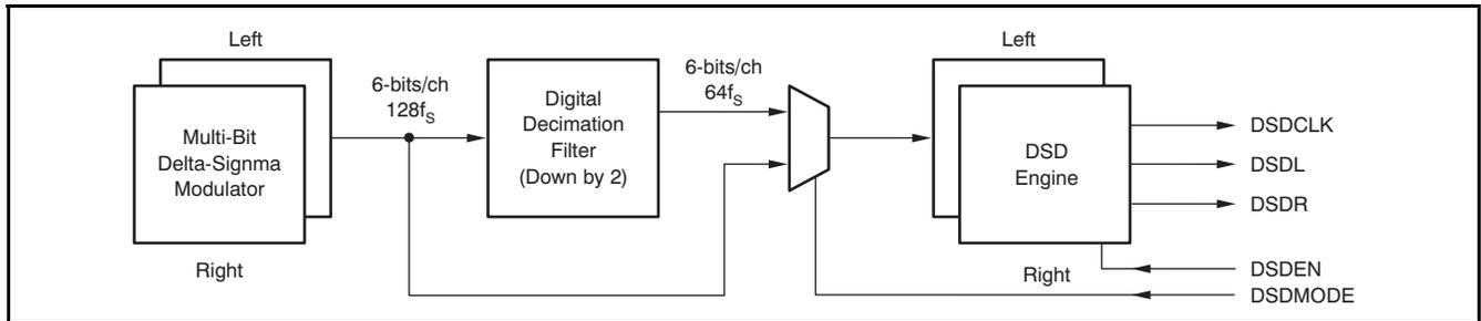
**Figure 46. Simplified Block Diagram for DSD Mode Operation**
