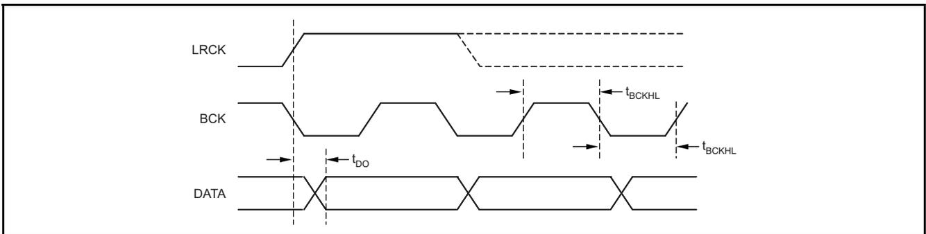
**Figure 2. Audio Serial Port Timing: TDM Data Formats**
