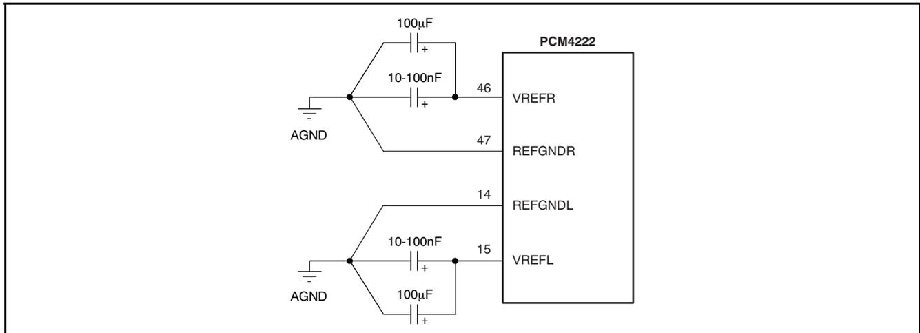
Figure 38. Recommended Reference Capacitor Connections and Values
