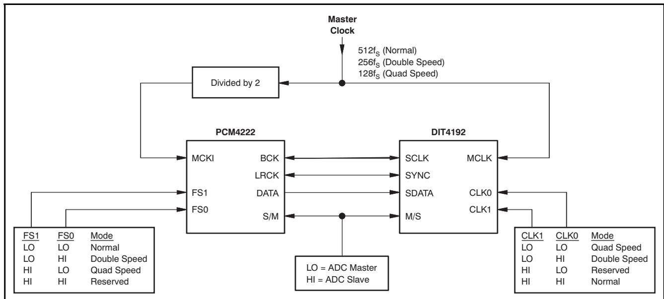
**Figure 53. Interfacing the PCM4222 to a [DIT4192](#)**
