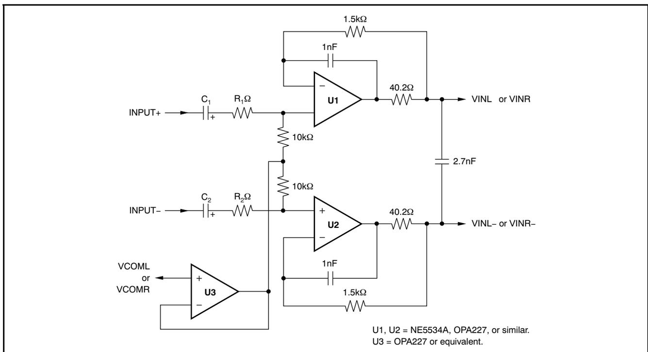
R<sub>1</sub> and R<sub>2</sub> are optional. When used, values may be selected for the desired attenuation.
