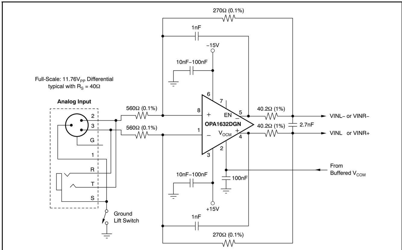
**Figure 50. Differential Input Buffer Circuit Utilizing the OPA1632**
