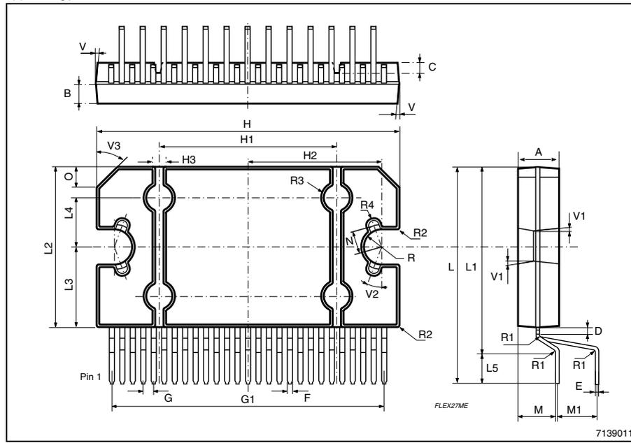
Figure 5. Flexiwatt27 (SMD) mechanical data and package dimensions
