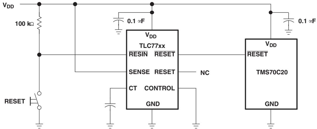
Figure 10. Reset Controller in a Microcomputer System
