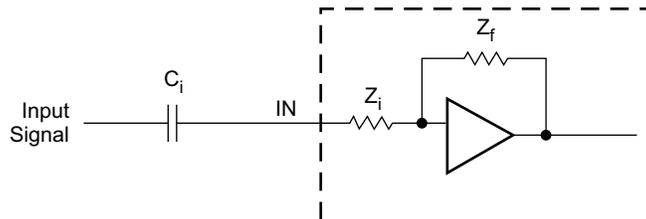
**Figure 26. Input Impedance**
