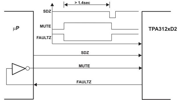
Figure 29. Timing Requirement for SDZ
