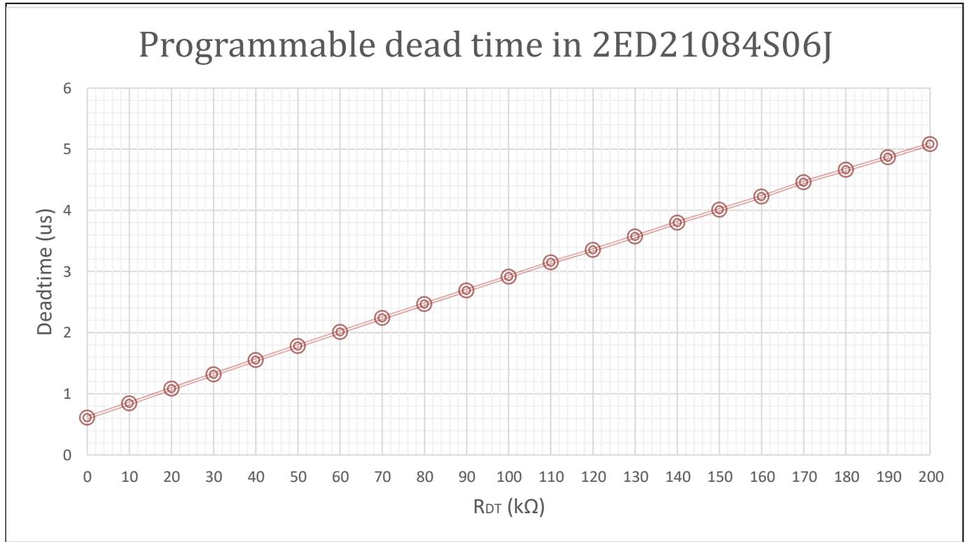
Figure 10 Variation of dead time vs. external resistor ( $R_{DT}$ )
