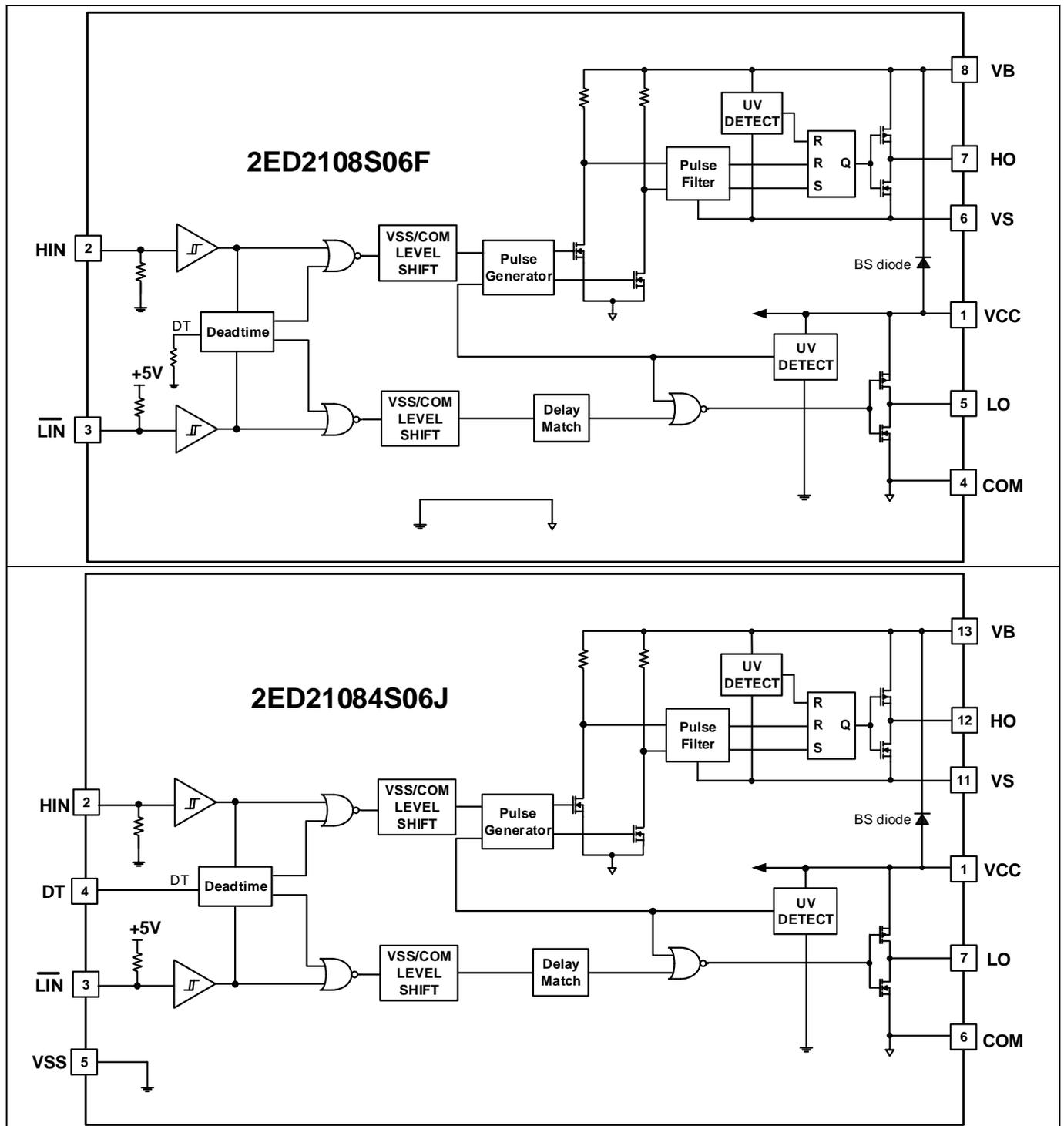
Figure 2 Block diagrams
