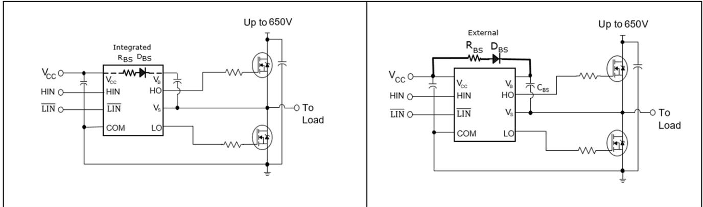
Figure 14 2ED210x with integrated components
