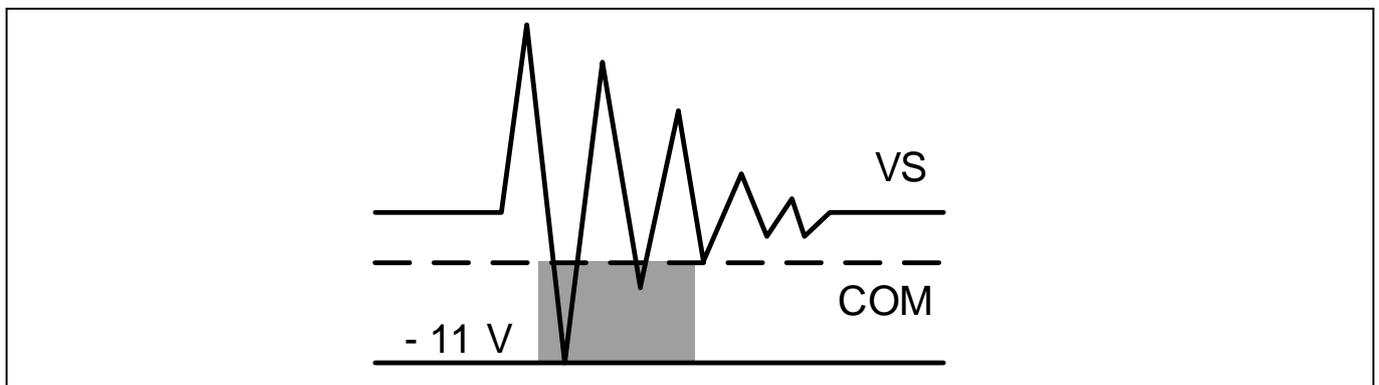
**Figure 22 Headroom for HV level shifter data transmission**
