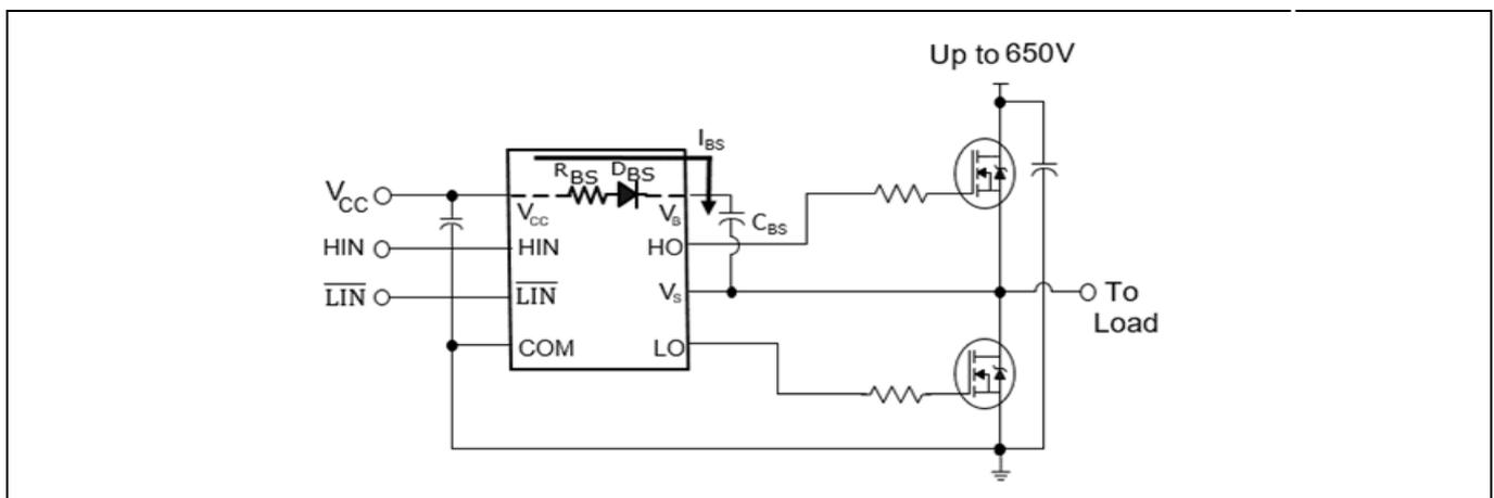
Figure 16 Half bridge bootstrap circuit in 2ED210x
