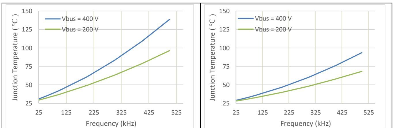
\*Assumptions for above curves: LLC topology, Power switch = IPP60R600P6,  $T_a = 25\text{ }^\circ\text{C}$ ,  $V_{BUS} = 400\text{ V}$ ,  $V_{CC} = 12\text{ V}$ ,  $R_{gon} = 3.9\ \Omega$ ,  $R_{goff} = 1\ \Omega$
