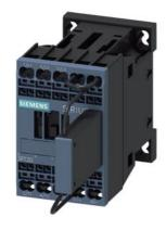
traction contactor, AC-3 12 A, 5.5 kW / 400 V 125 V DC, 0.7-1.25\*US with integrated suppressor diode 3-pole, size S00 spring-type terminal suitable for PLC outputs not expandable with auxiliary switch
