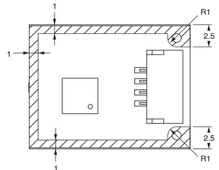
Note: Due to insulation distance limitations, do not allow metal parts to come into contact with the Sensor.
