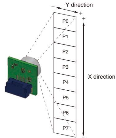
Note: Definition of view angle: Using the maximum Sensor output as a reference, the angular range where the Sensor output is 50% or higher when the angle of the Sensor is changed is defined as the view angle.
