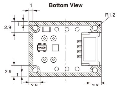
Note: Due to insulation distance limitations, do not allow metal parts to come into contact with the Sensor.
