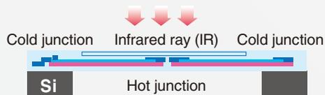
The sensor utilizes the seebeck effect in which thermoelectric force is generated due to the temperature difference that occurs across the junction points of two different types of metal.
