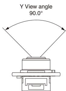
Note: Definition of view angle: Using the maximum Sensor output as a reference, the angular range where the Sensor output is 50% or higher when the angle of the Sensor is changed is defined as the view angle.
