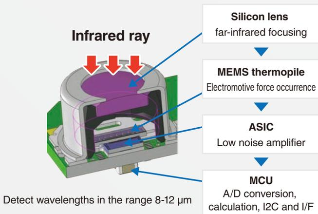
**MEMS thermopile detection principle**
