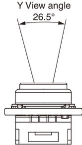
Note: Definition of view angle: Using the maximum Sensor output as a reference, the angular range where the Sensor output is 50% or higher when the angle of the Sensor is changed is defined as the view angle.
