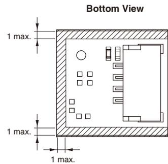
Note: Due to insulation distance limitations, do not allow metal parts to come into contact with the Sensor.
