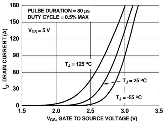
**Figure 5. Transfer Characteristics**
