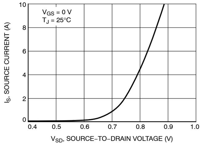
Figure 10. Diode Source Current vs. Forward Voltage
