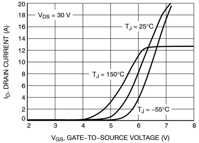
Figure 2. Transfer Characteristics
