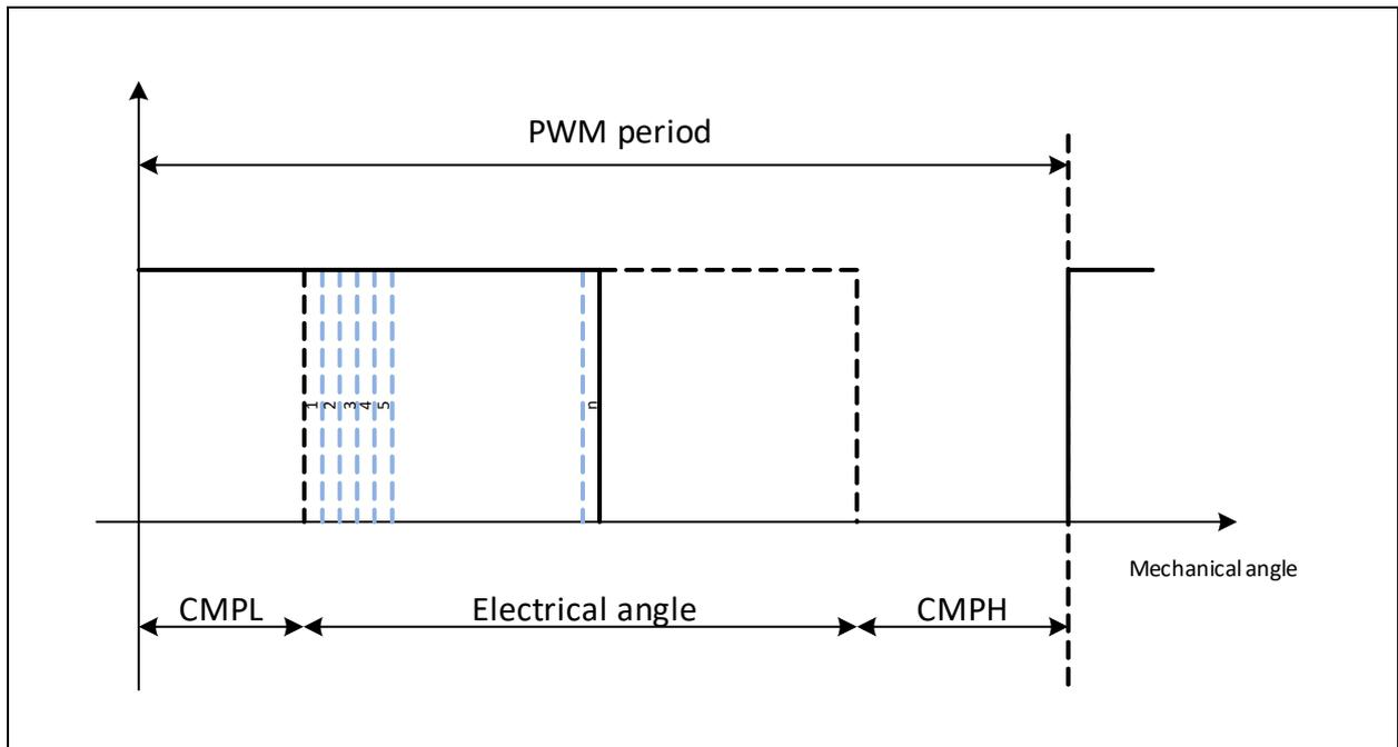
The [PWMFR](#) setting sets the duration of the PWM frequency. The [PWMSR](#) setting chooses between fast and slow steps.
