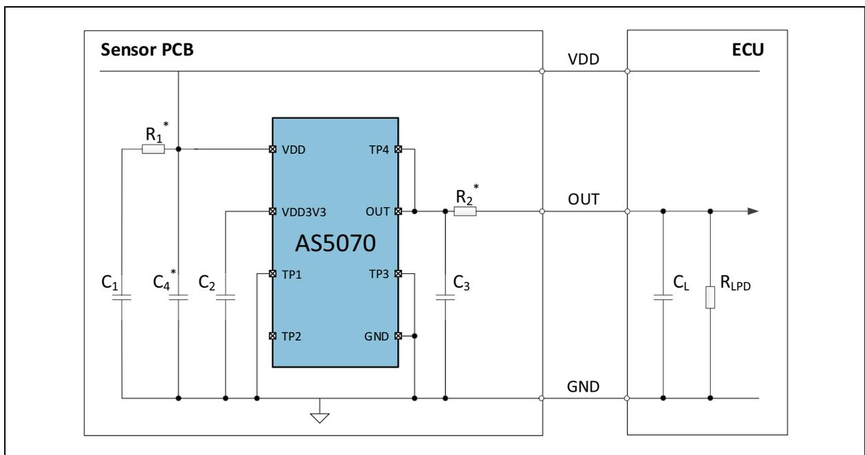
Figure 43 and Figure 44 show the recommended schematic in the application. All components marked with (\*) are optional and can be used to further increase the EMC.
