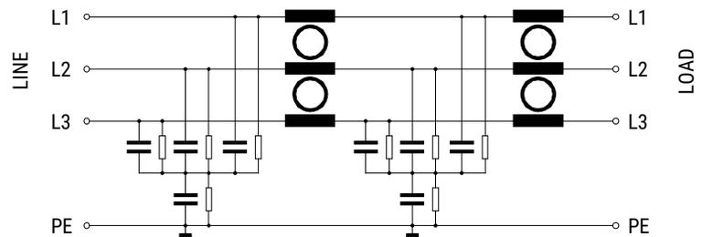
\* Maximum leakage current under normal operating conditions. If two phases are interrupted, leakage current can be much higher. Filters without Y capacitors have no leakage current.
