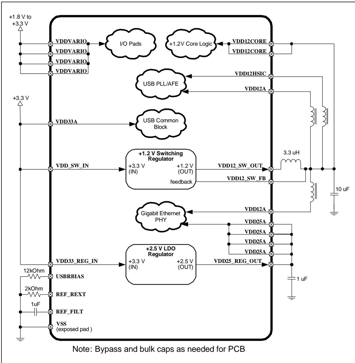
**Note:** For 3.3V I/O operation, the **VDDVARIO** and +3.3V supplies may be connected together. To disable the internal switcher, tie the **VDD12\_SW\_FB** pin to 3.30V and ensure that all **VDD12** rails are connected to an external 1.20V supply.
