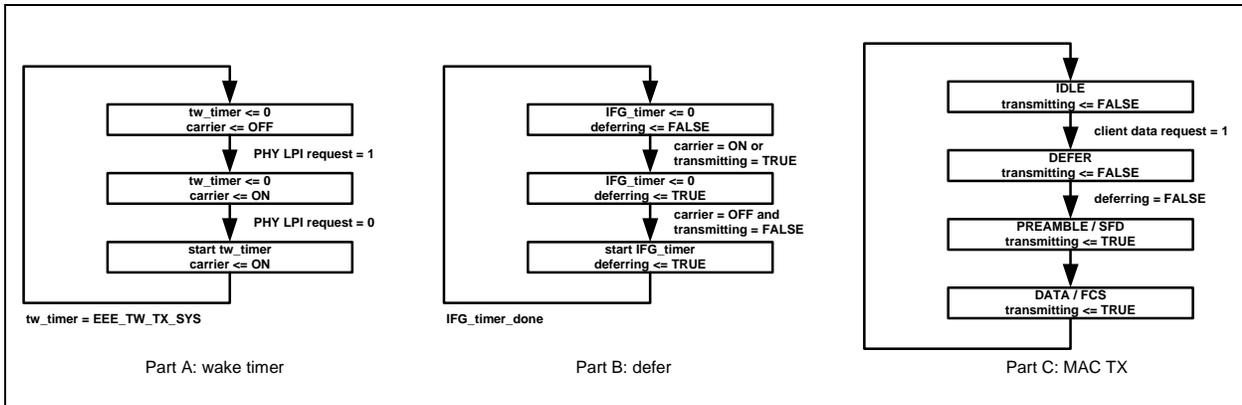
In part A of the figure, a carrier indicator is set when the TX LPI request to the PHY is asserted. The wake timer (`tw_timer`) is triggered when the TX LPI request to the PHY is de-asserted and once the wake timer is satisfied, the carrier indicator is cleared. Note that there are separate TX wait values depending on the speed of operation.
