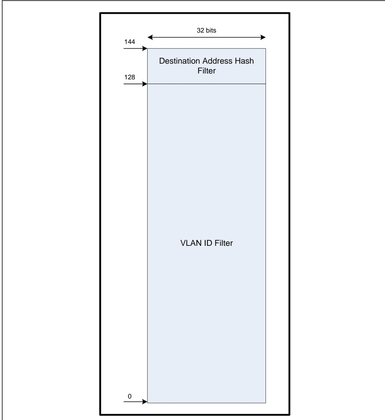
VHF entries are added and changed via the data port registers. The [Data Port Select Register \(DP\\_SEL\)](#) is used to specify the VHF RAM. The VHF entries may be changed during run time.
