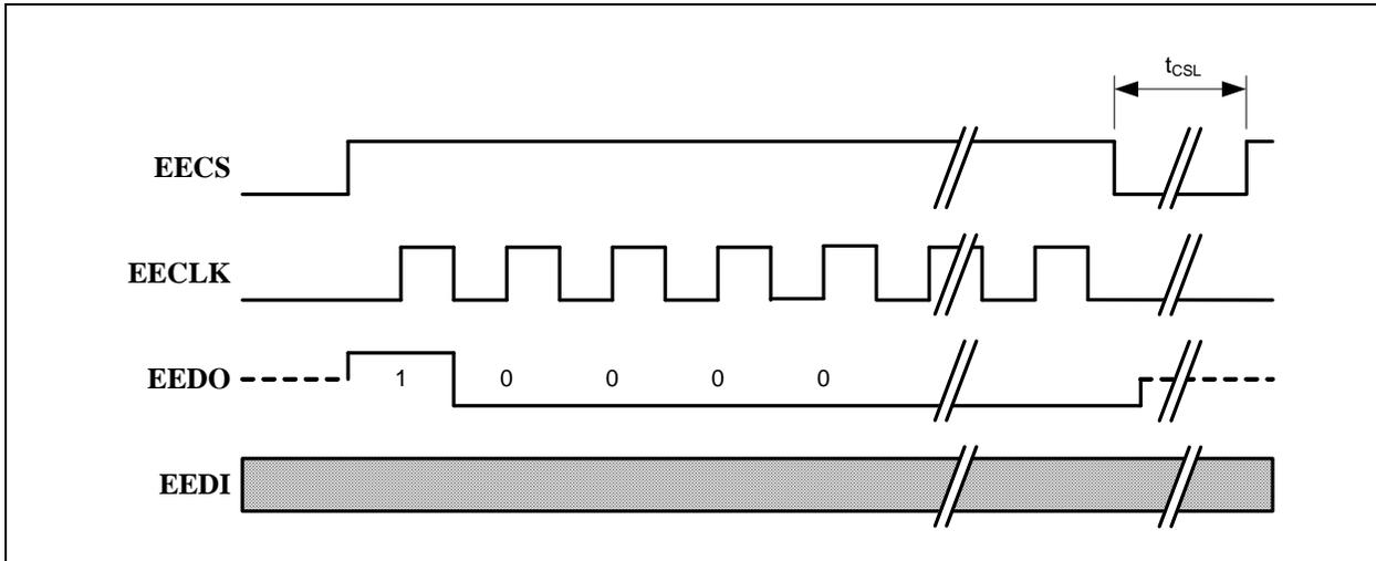
**EWEN (Erase/Write Enable):** Enables the EEPROM for erase and write operations. The EEPROM will allow erase and write operations until the "Erase/Write Disable" command is sent, or until power is cycled.
