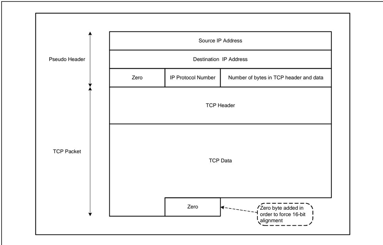
FIGURE 7-8: TCP CHECKSUM - IPV6
