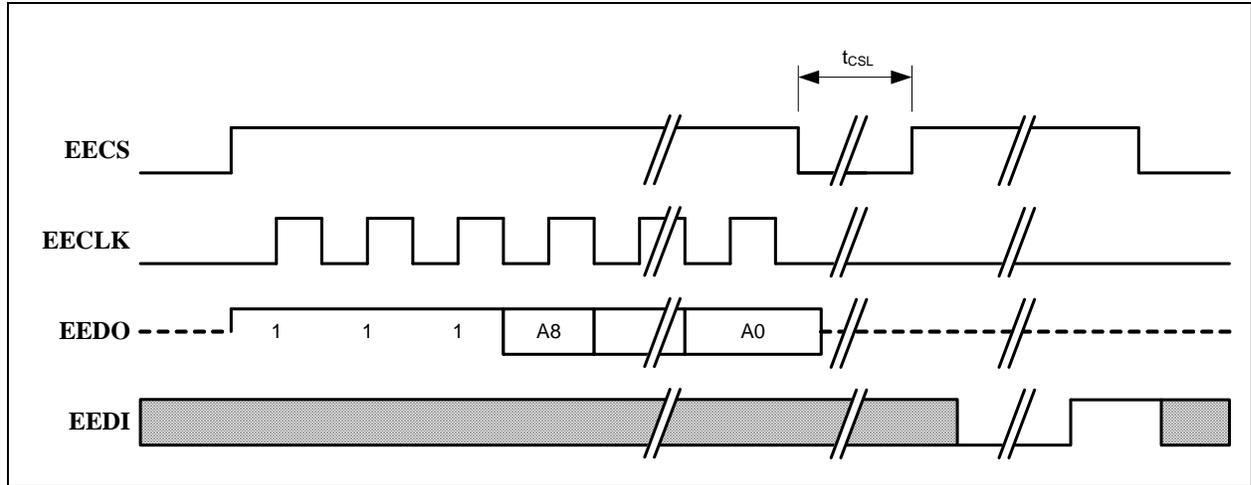
**ERASE (Erase All):** If erase/write operations are enabled in the EEPROM, this command will initiate a bulk erase of the entire EEPROM. The EPC\_TO bit is set if the EEPROM does not respond within 30 ms.
