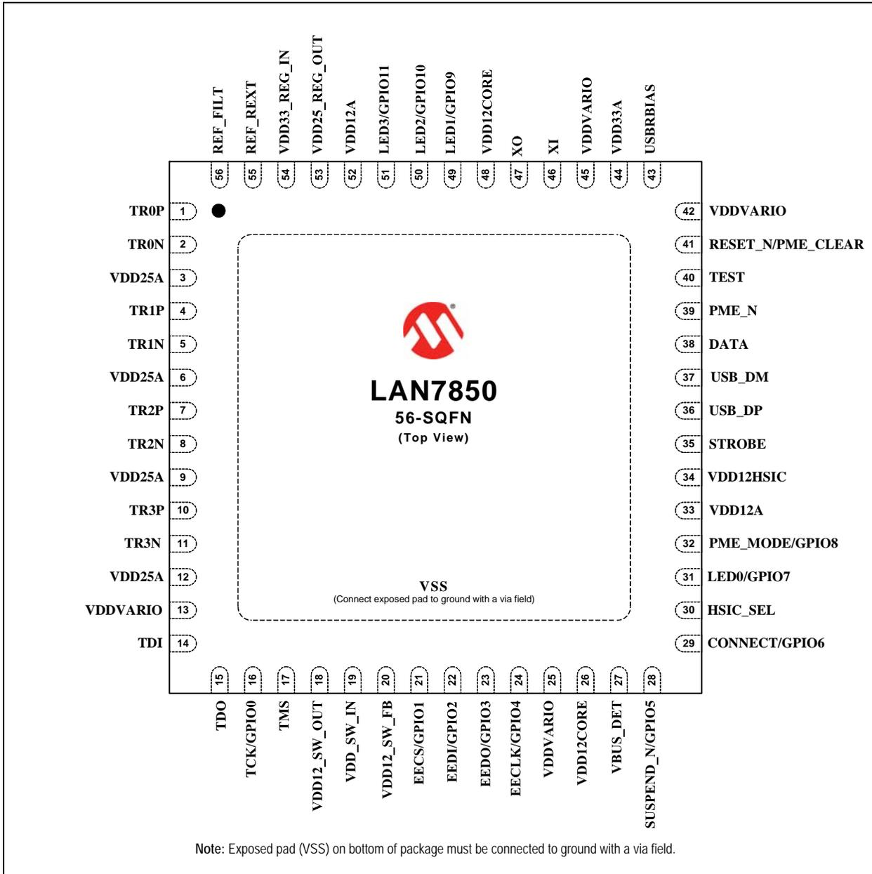
**Note:** When an “\_N” is used at the end of the signal name, it indicates that the signal is active low. For example, RESET\_N indicates that the reset signal is active low.
