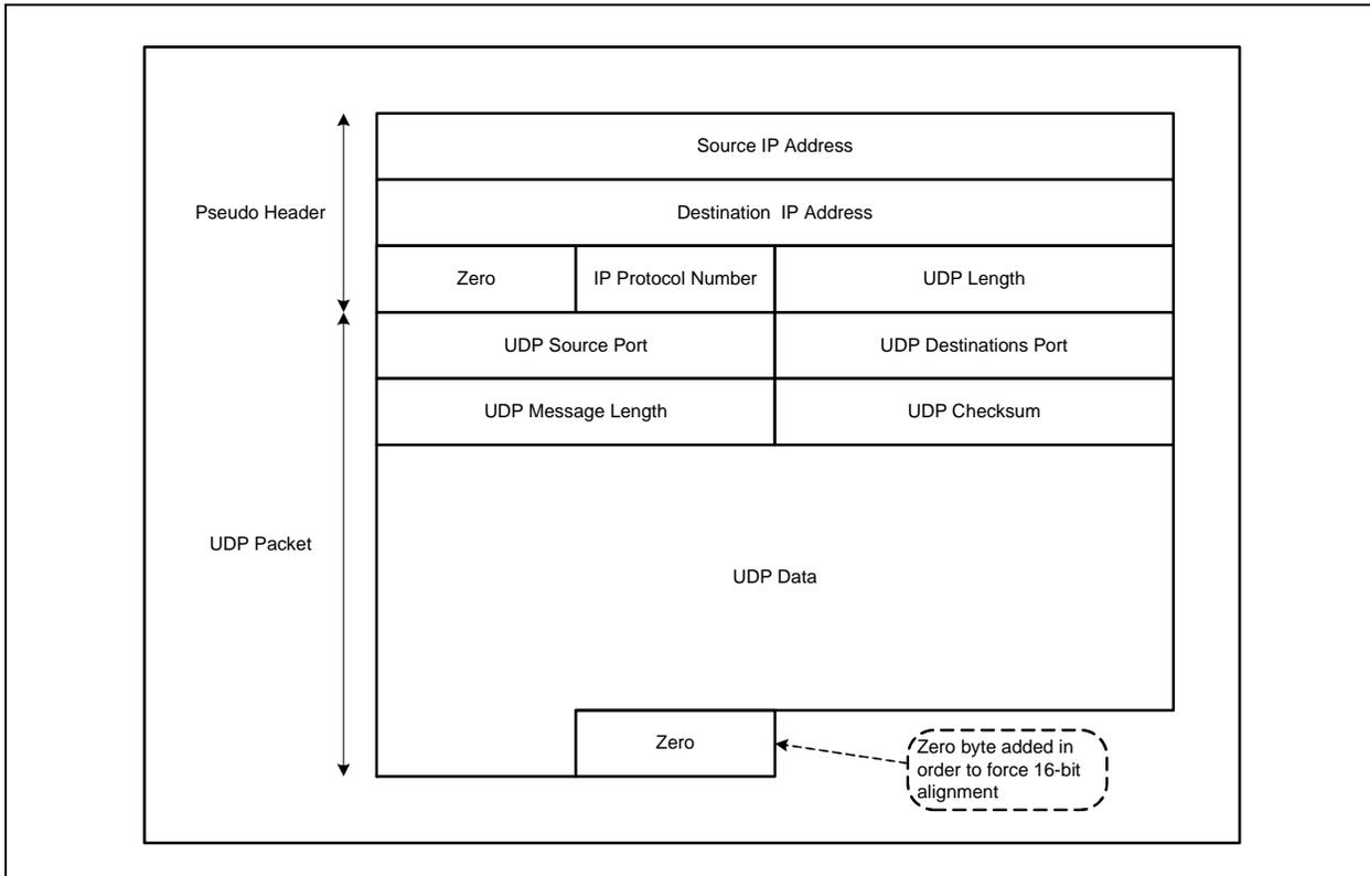
**FIGURE 7-10: UDP CHECKSUM - IPV6**
