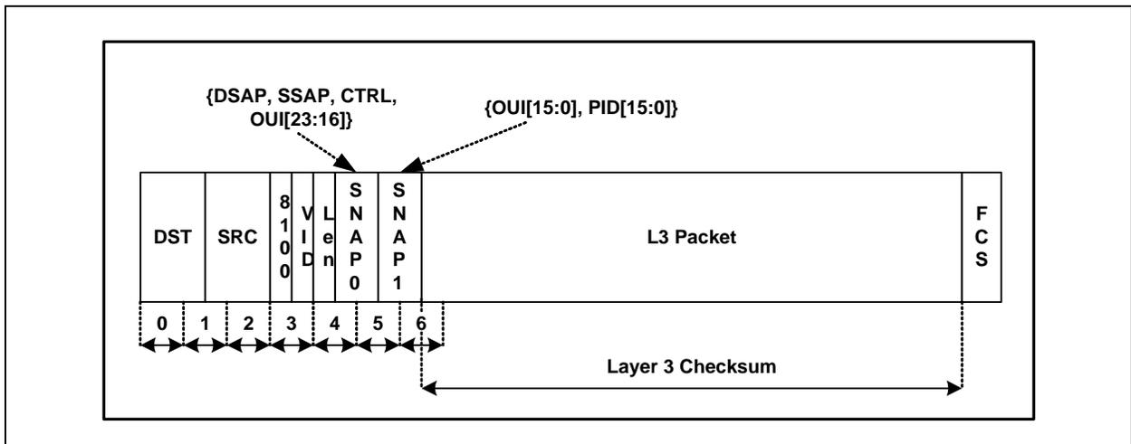
The checksum is placed in the [Raw L3 Checksum](#) field in [RX Command B](#). This raw checksum is useful in cases such as when the layer 3 protocol is not IP or IP fragmented packets.
