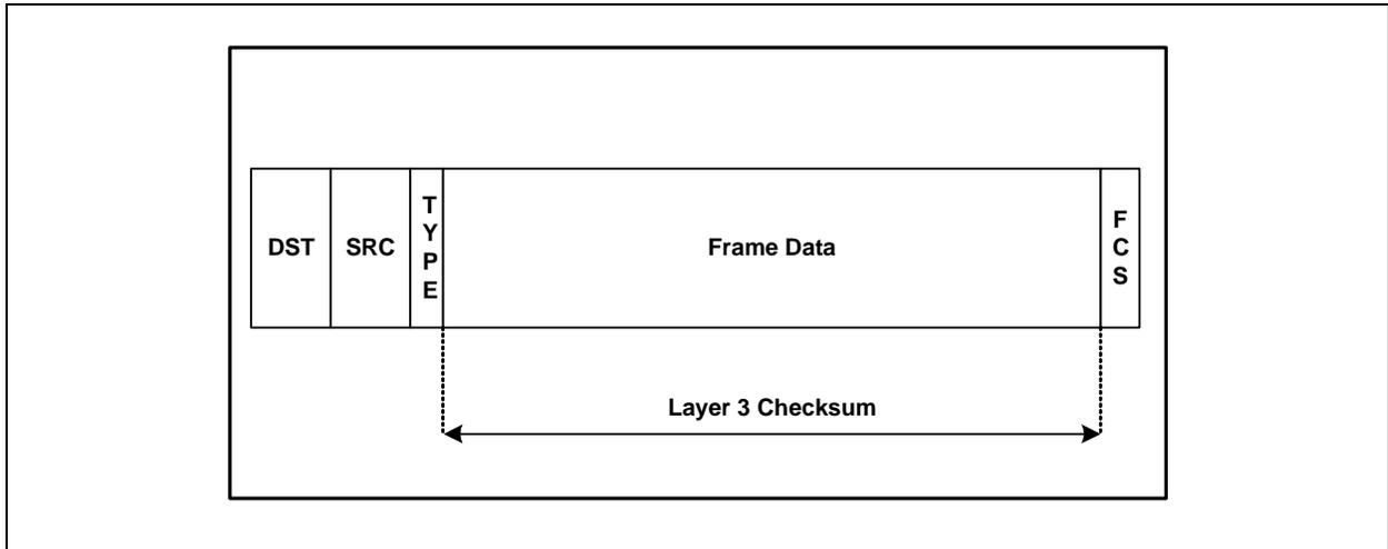
Consider the case where the frame is a 802.3 Ethernet frame with a VLAN tag. The RFE bypasses DA, SA, VLAN tag, SNAP header, and type fields. The calculation begins at the byte immediately following the type field. The calculation does not include the FCS.
