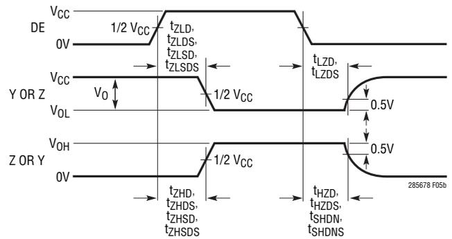
Figure 5. Driver Enable and Disable Timing Measurement
