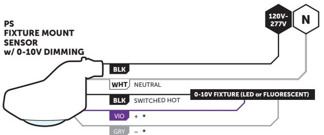
\* VIO/GRY DIMMING WIRES (0-10V) SHOULD BE TREATED AS CLASS 1
