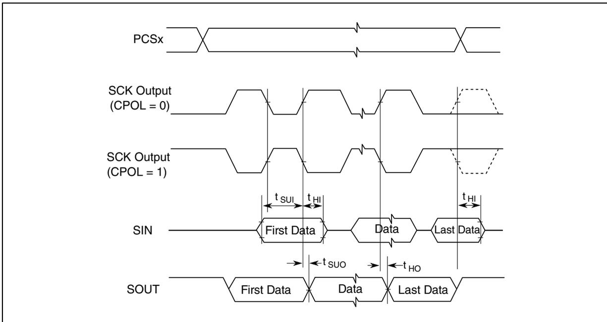
Figure 36. DSPI CMOS master mode – modified timing, CPHA = 1
