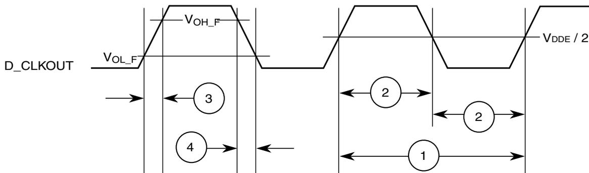
**Figure 25. D\_CLKOUT timing**
