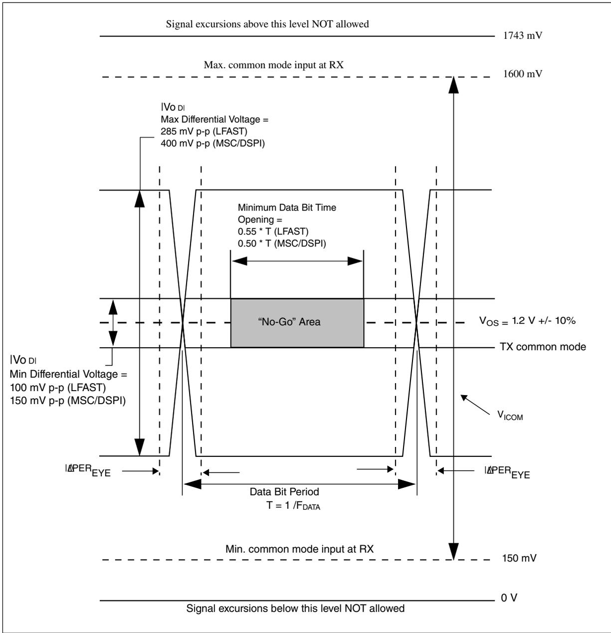
Figure 8. LFAST and MSC/DSPI LVDS timing definition
