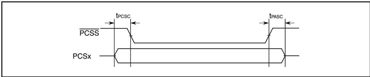
Figure 37. DSPI PCS strobe ( $\overline{\text{PCSS}}$ ) timing (master mode)
