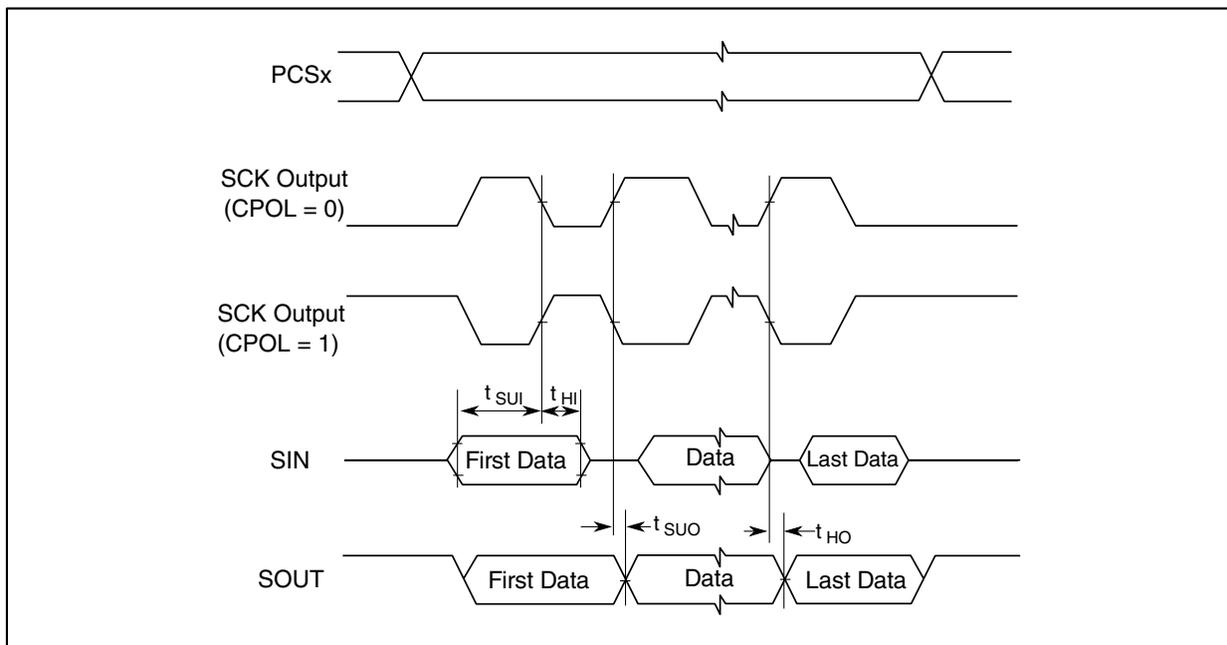
**Figure 33. DSPI CMOS master mode – classic timing, CPHA = 1**
