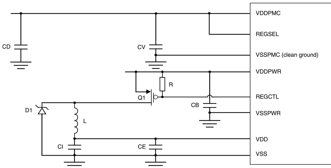
**Figure 13. SMPS configuration****NOTE**
