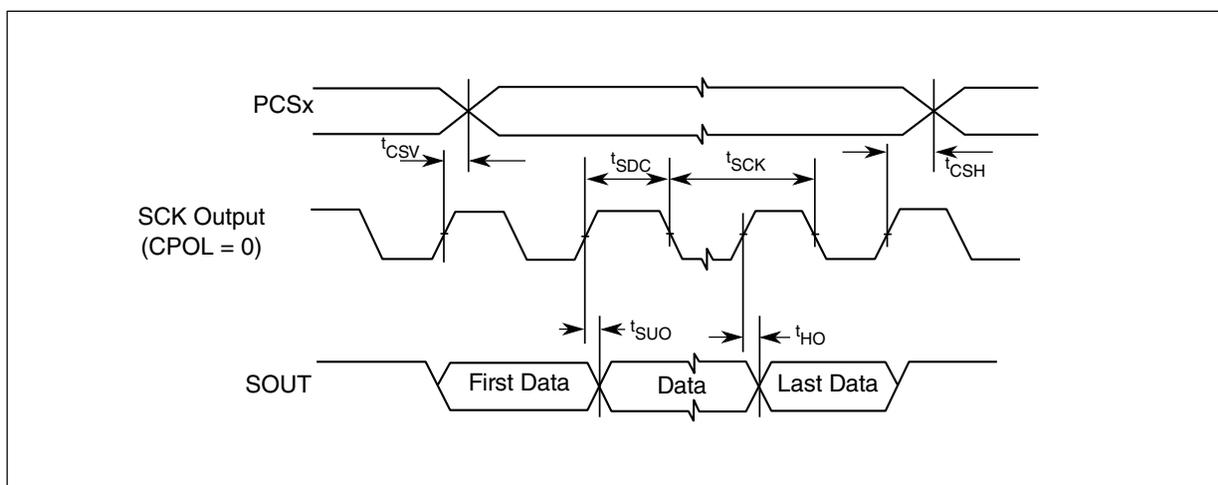
**Figure 40. DSPI LVDS and CMOS master timing – output only – modified transfer format
