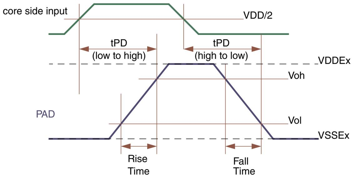
**Figure 5. I/O output DC electrical characteristics definition**
