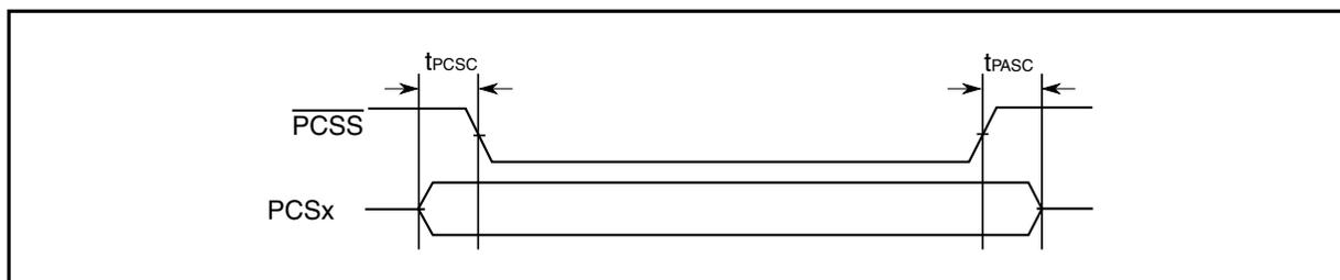
Figure 34. DSPI PCS strobe ( $\overline{\text{PCSS}}$ ) timing (master mode)
