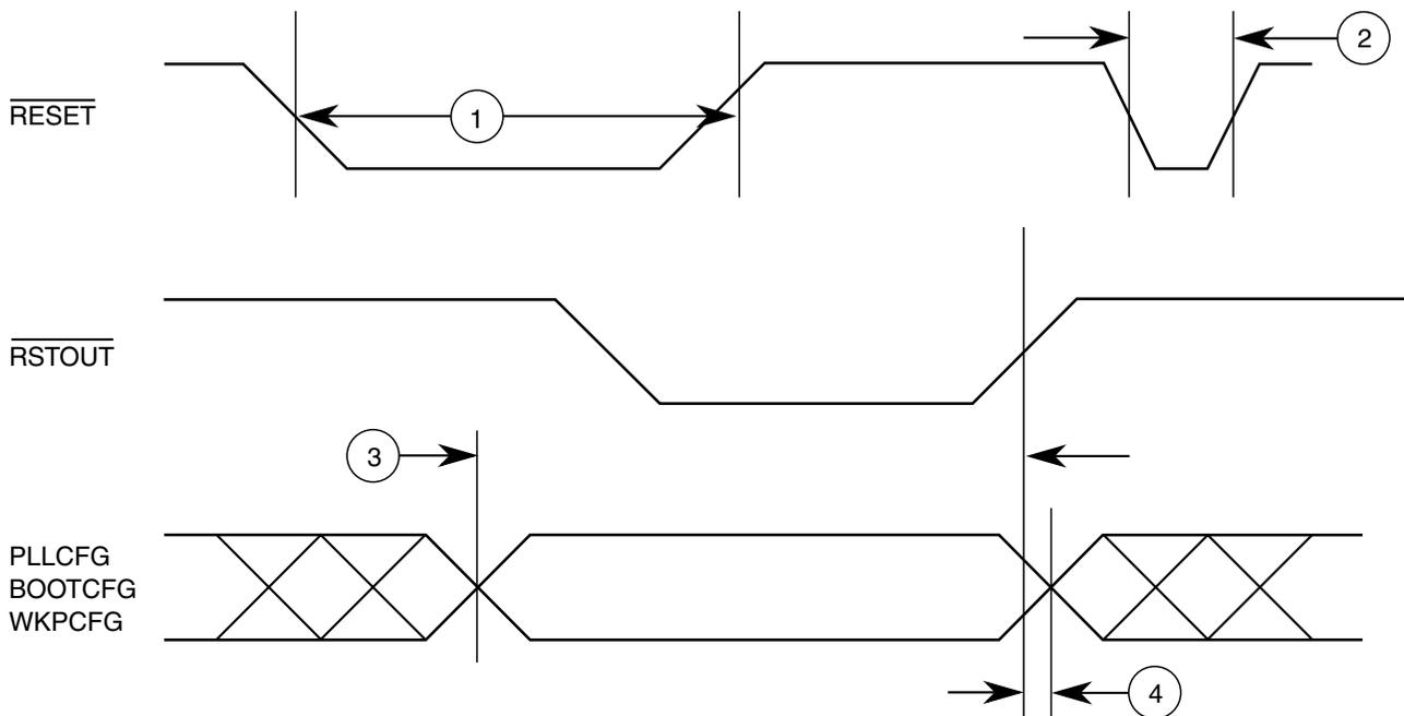
Figure 18. Reset and configuration pin timing
