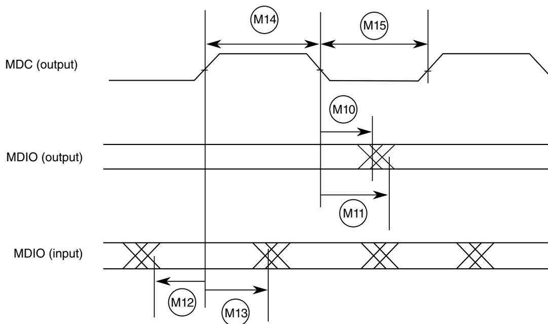
**Figure 46. MII serial management channel timing diagram**
