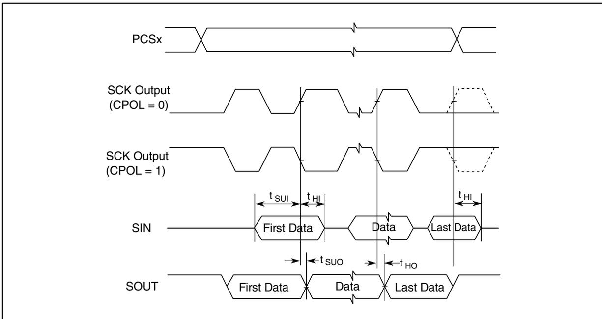
Figure 39. DSPI LVDS master mode – modified timing, CPHA = 1
