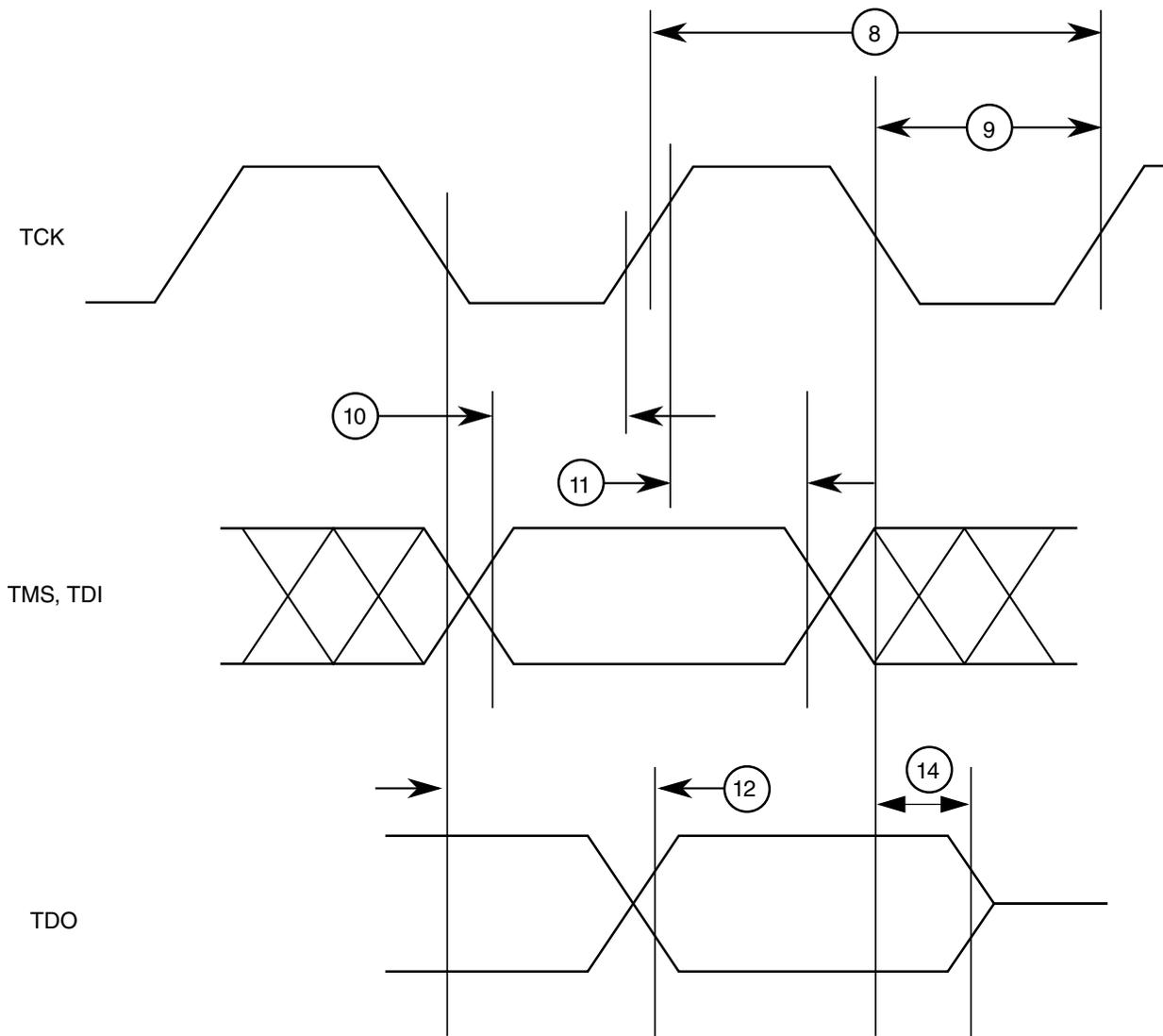
Figure 24. Nexus TCK, TDI, TMS, TDO Timing
