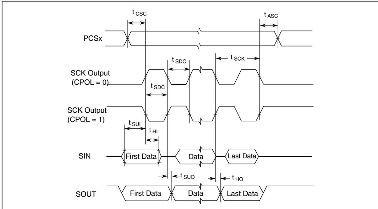
**Figure 32. DSPI CMOS master mode – classic timing, CPHA = 0**
