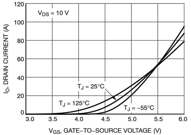
Figure 2. Transfer Characteristics
