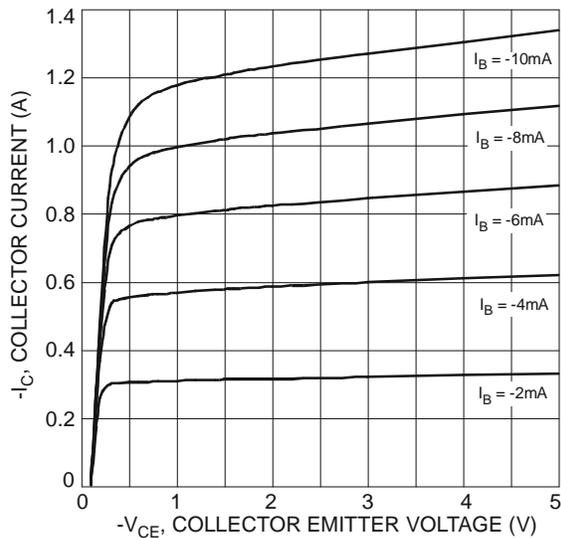
Figure 1. Typical Collector Current vs. Collector-Emitter Voltage
