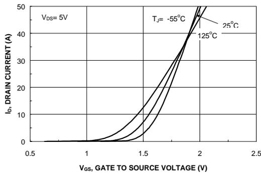
Figure 5. Transfer Characteristics.
