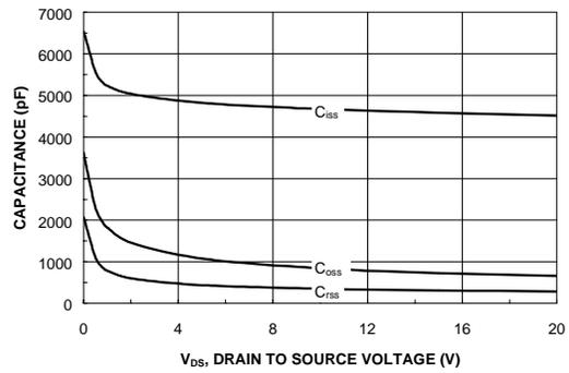
**Figure 8. Capacitance Characteristics.**
