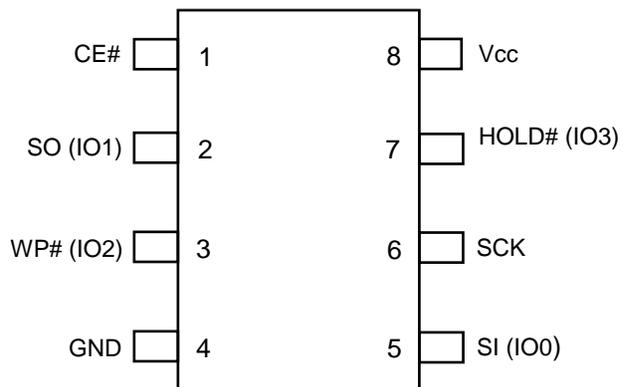
8-pin SOIC 208mil (Package: B)
