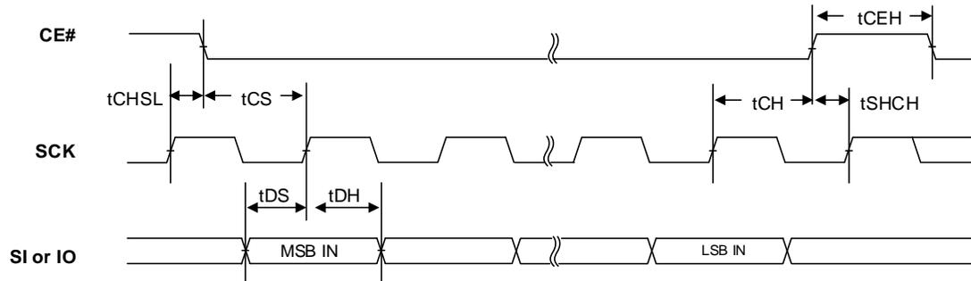
Figure 9.3 SERIAL INPUT TIMING (DTR Mode)
