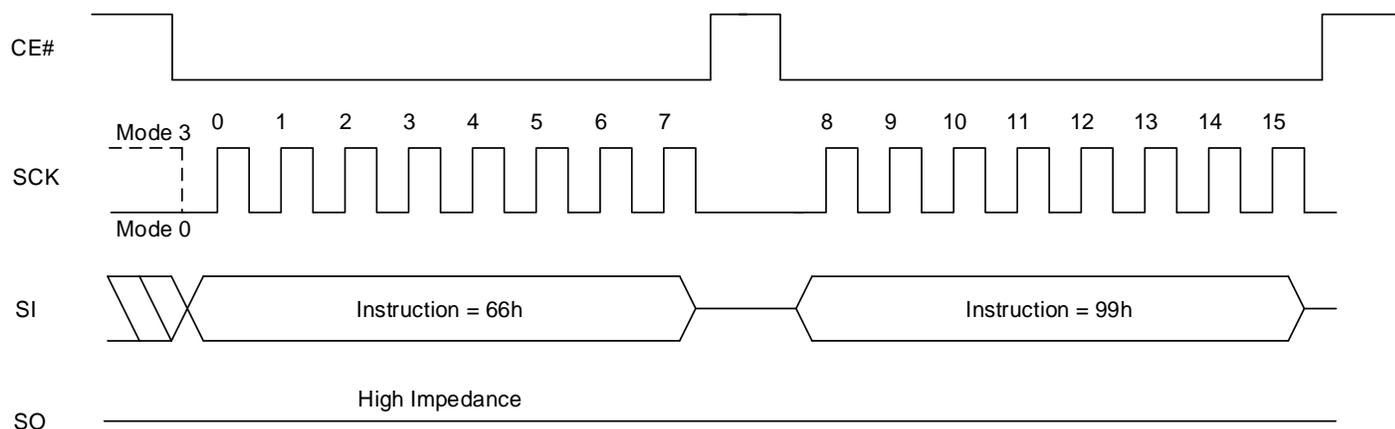
**Figure 8.51 Software Reset Enable and Software Reset Sequence In QPI Mode (RSTEN, 66h + RST, 99h)**
