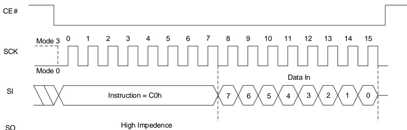
Figure 8.41 Set Wrapped Burst Read Sequence In QPI Mode
