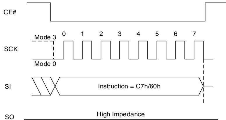
**Figure 8.21 Chip Erase Sequence In QPI Mode**
