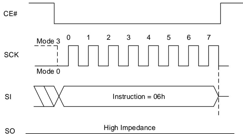
**Figure 8.23 Write Enable Sequence In QPI Mode**
