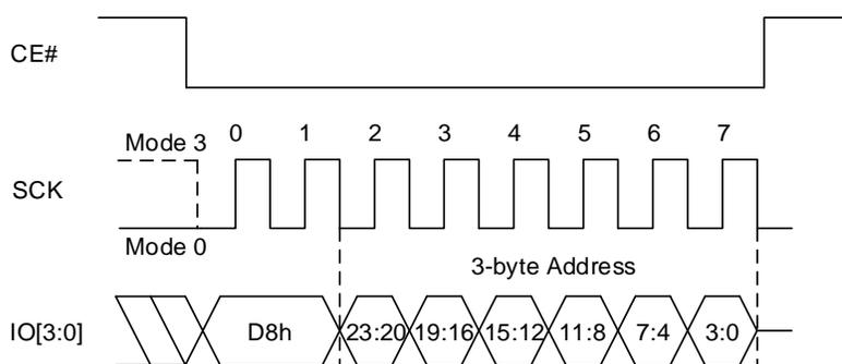
Figure 8.18 Block Erase (32KB) Sequence In SPI Mode
