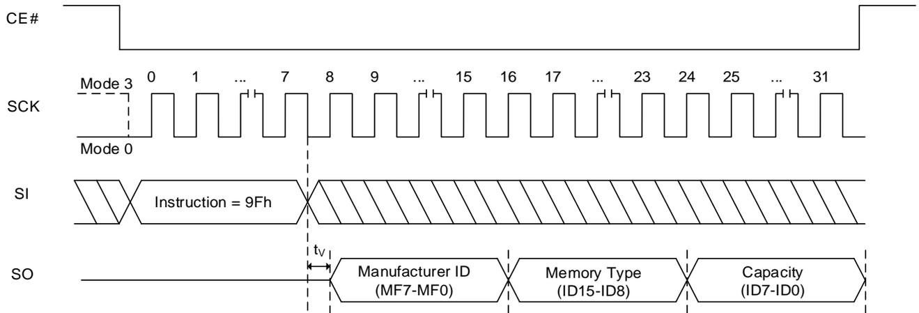
**Figure 8.45 RDJDID and RDJDIDQ DJJDIDQ (Read JEDEC ID In QPI Mode) Sequence**
