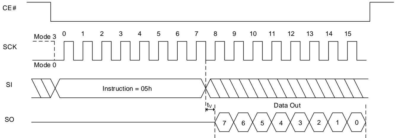
**Figure 8.27 Read Status Register Sequence In QPI Mode**
