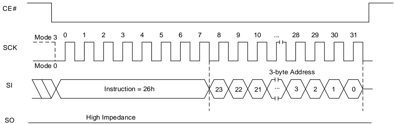
**Figure 8.56 Sector Unlock QPI Sequence In QPI Mode**
