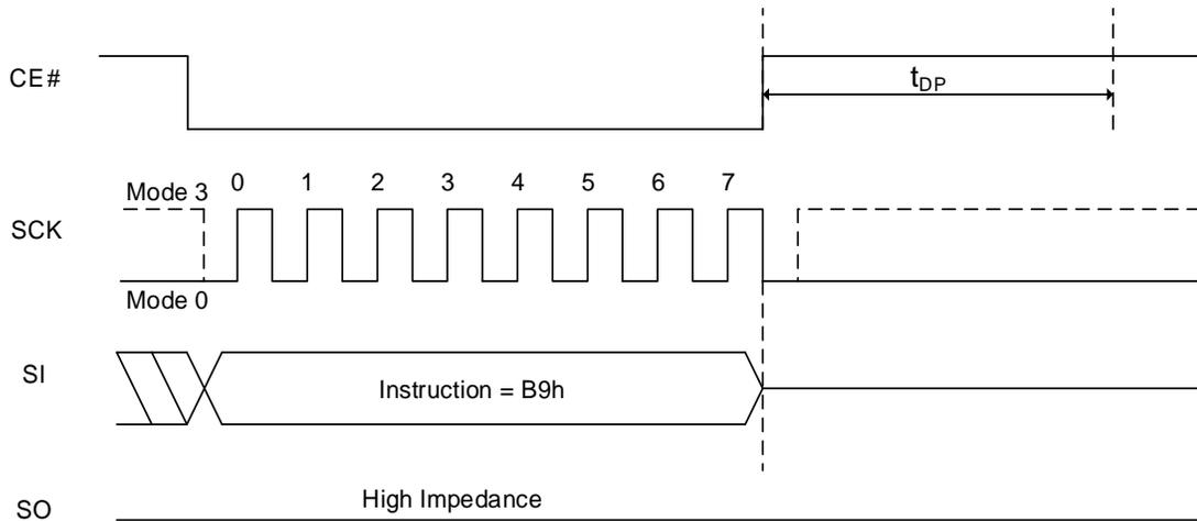
**Figure 8.37 Enter Deep Power Down Mode Sequence In QPI Mode**
