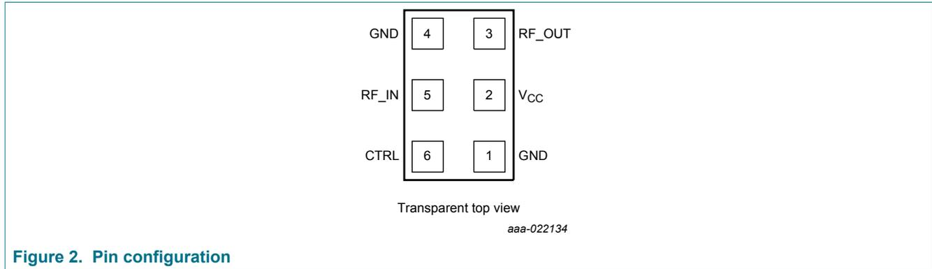
Figure 2. Pin configuration
