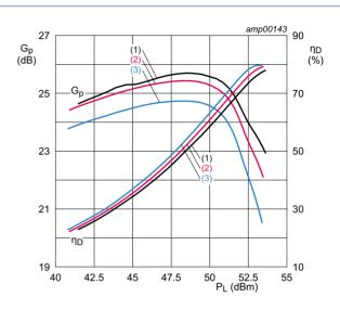
$V_{DS}$  = 28 V;  $I_{Dq}$  = 350 mA.
