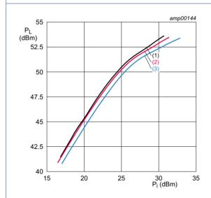
$V_{DS}$  = 28 V;  $I_{Dq}$  = 350 mA.
