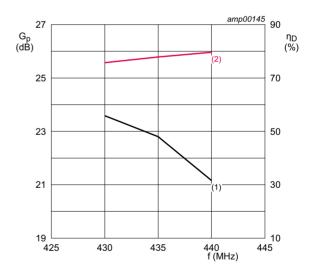
$V_{DS}$  = 28 V;  $I_{Dq}$  = 350 mA;  $P_{L}$  = 200 W
