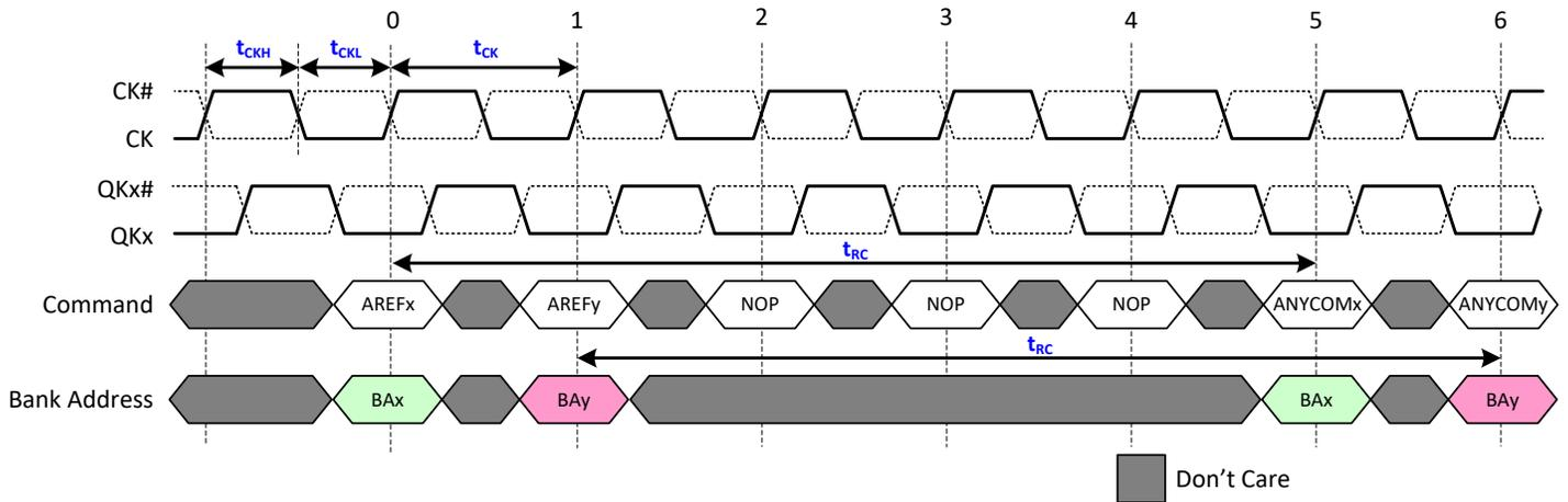
**AREF example in t<sub>RC</sub>(t<sub>CK</sub>)=5 option: Configuration=5**
