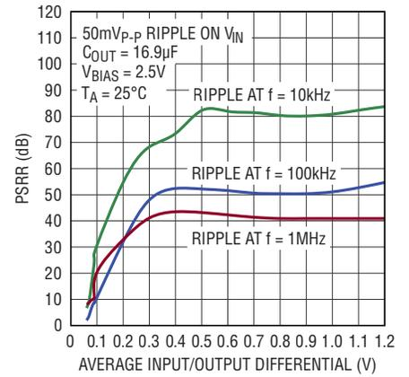
**IN Pin Ripple Rejection vs  $V_{IN} - V_{OUT}$ , 1V/1A**
