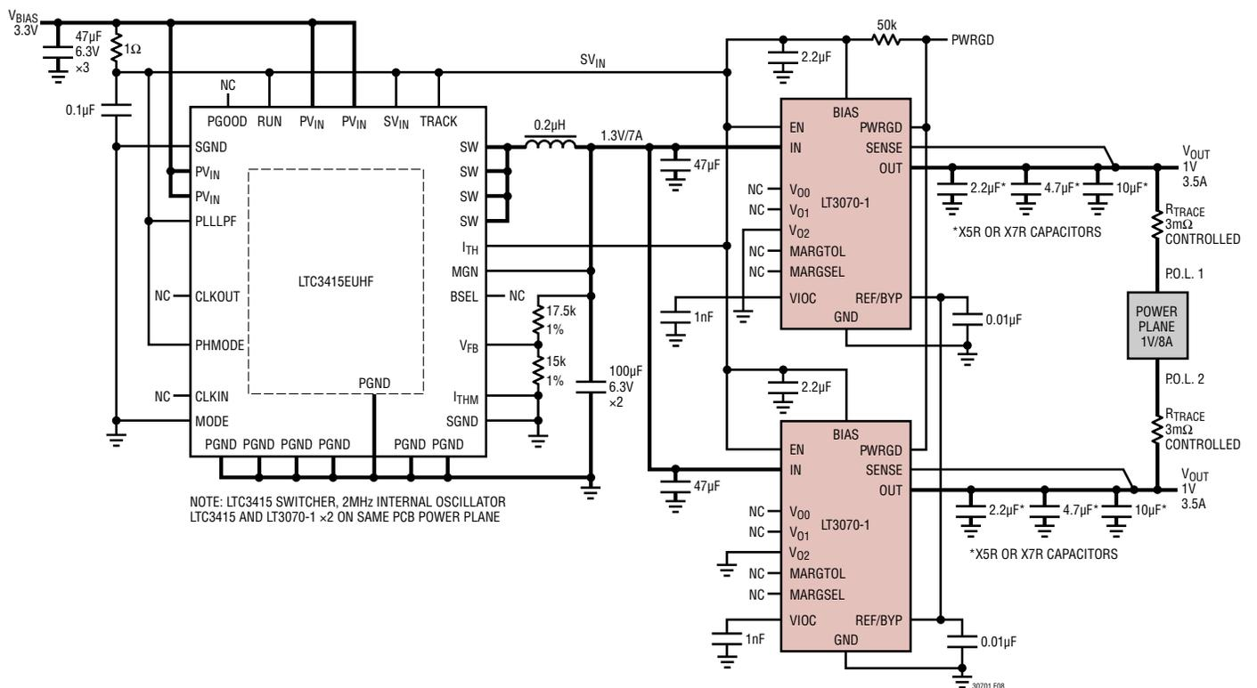
Figure 8. 1V, 7A Point-of-Load Current Sharing Regulators
