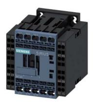
power contactor, AC-3 12 A, 5.5 kW / 400 V 1 NC, 110 V DC, with diode integrated, 3-pole Size S00, Spring-type terminal 3RH2921-2DA11 (1 NO + 1 NC) mounted left and right
