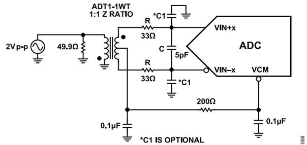
**Figure 59. Differential Transformer-Coupled Configuration for Baseband Applications**
