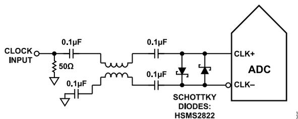
Figure 63. Balun-Coupled Differential Clock (Up to 1 GHz)
