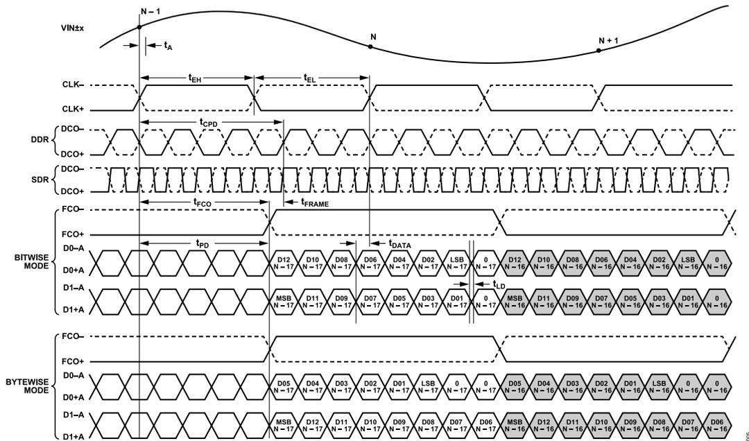
Figure 4. 16-Bit DDR/SDR, Two-Lane, 2x Frame Mode
