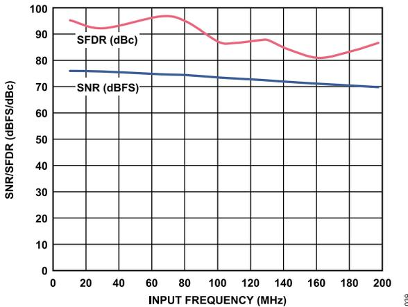
Figure 18. SNR/SFDR vs.  $f_{IN}$ ,  $f_{SAMPLE} = 80$  MSPS
