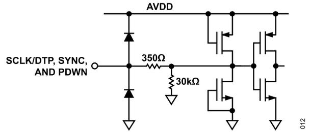
Figure 51. Equivalent SCLK/DTP, SYNC, and PDWN Input Circuit
