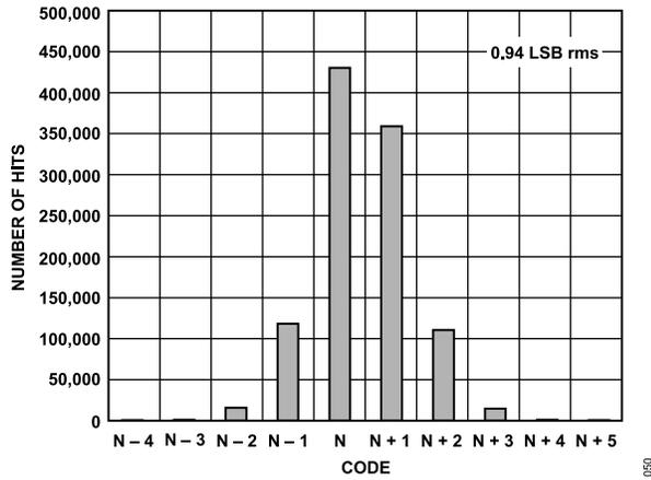
Figure 43. Input-Referred Noise Histogram,  $f_{SAMPLE} = 125 \text{ MSPS}$
