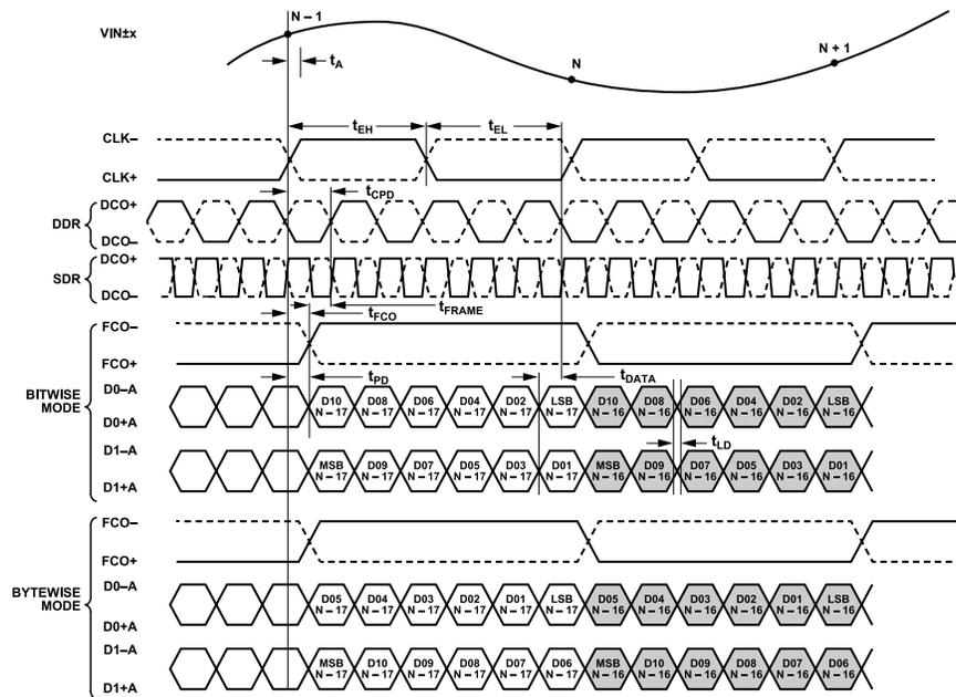
Figure 5. 12-Bit DDR/SDR, Two-Lane, 2x Frame Mode
