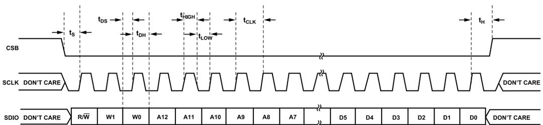
**Figure 74. Serial Port Interface Timing Diagram**
