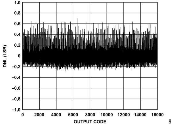
Figure 42. DNL,  $f_{IN} = 9.7 \text{ MHz}$ ,  $f_{SAMPLE} = 125 \text{ MSPS}$
