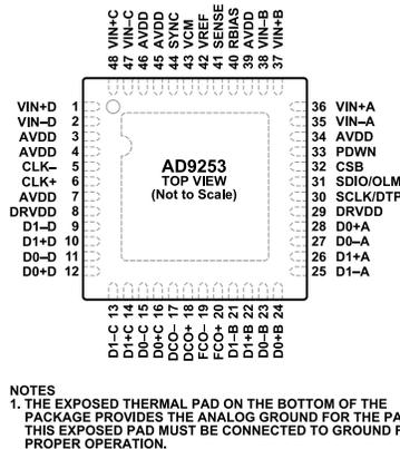
Figure 9. 48-Lead LFCSP Pin Configuration, Top View
