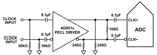
Figure 65. Differential PECL Sample Clock (Up to 1 GHz)
