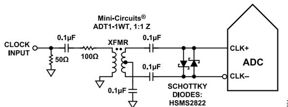
Figure 62. Transformer-Coupled Differential Clock (Up to 200 MHz)
