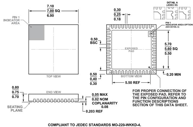
**Figure 77. 48-Lead Lead Frame Chip Scale Package [LFCSP]
