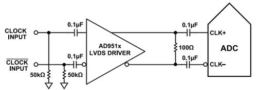
Figure 66. Differential LVDS Sample Clock (Up to 1 GHz)
