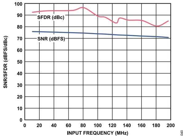
Figure 28. SNR/SFDR vs.  $f_{IN}$ ,  $f_{SAMPLE} = 105$  MSPS
