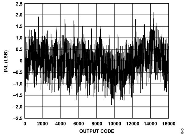
Figure 41. INL,  $f_{IN} = 9.7 \text{ MHz}$ ,  $f_{SAMPLE} = 125 \text{ MSPS}$
