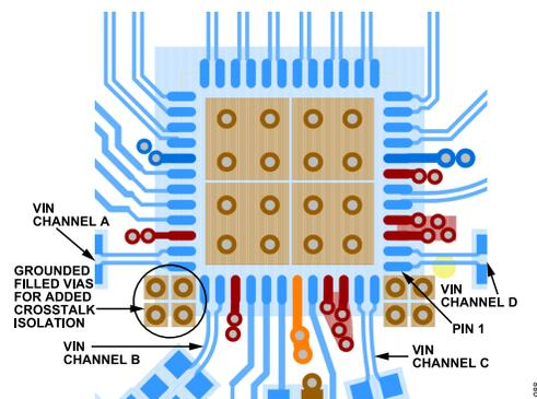
Figure 76. Layout Technique to Maximize Crosstalk Performance
