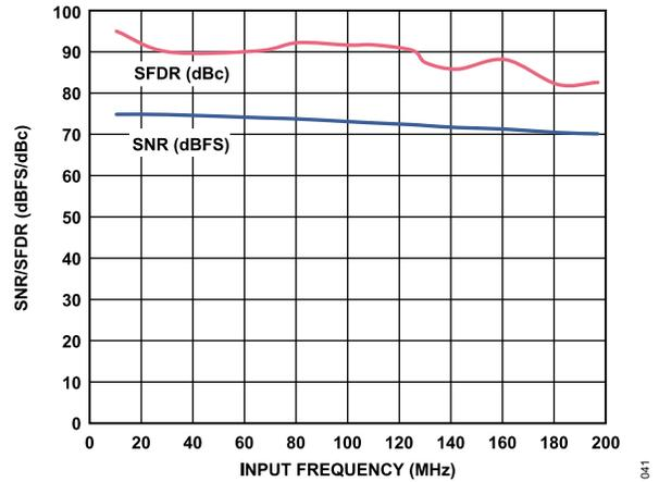
Figure 39. SNR/SFDR vs.  $f_{IN}$ ,  $f_{SAMPLE} = 125 \text{ MSPS}$
