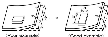
(2) Components location on PCB separation
